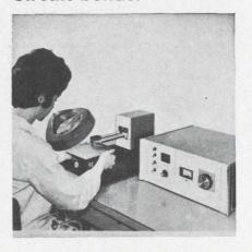
The model 730 bonder uses infrared detection and bonds components and wiring in assemblies, to PC cards or to thin films. It welds, brazes, hard and soft solders and bonds using parallel gap or opposed heads. Temperatures from 300°F to 1400°F are controlled so that, once bonding mode and temperature are selected operation is automatic. The power supply has a capacity of 500 A at 2 V for 10 s.
