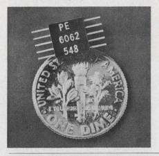
Microminiature transformers of this series can be used with sense amplifiers and discriminator circuitry and as common mode chokes. The "Flat-Tran" is compatible with ICs and standard flat pack connectors. Twelve designs are available from 25  $\mu$ H to 240  $\mu$ H. All models have gold-plated kovar leads to TO-91 packages.
