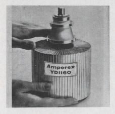
An axial ceramic, conical triode is for dielectric and industrial heating use. Rated to 160 MHz, the tube can be operated to 250 MHz when derated. As a class C oscillator, it will produce 8.2 kW at 82% efficiency, with a 5-kV plate voltage. The tube features thoriated tungsten mesh cathodes and mesh "K" grids. An integral radiator permits forced air cooling.
