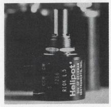
A wirewound, 10-turn pot has 7/8-in. diameter and is 3/4-in. long. Standard values are 10  $\Omega$  to 125 k $\Omega$ . Tolerance is  $\pm 3\%$  with  $\pm 0.2\%$  independent linearity.
