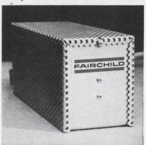
A solid-state plug-in replacement for popular tube-type amplifiers is announced. This amplifier, designated the A00-954, provides  $\pm$  40 mA at  $\pm$  100 V and  $\pm$  10 mA at 140 V. Applications are claimed in place of vacuum tube amplifiers to improve system reliability and avoid downtime. It operates directly on available  $\pm$ 300 V supplies.
