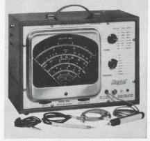
This VTVM features a 9-in. display and covers 0 to 1500 Vdc. Other ranges are 0 to 1500 mAdc, 0 to 1500 Vac rms and p-p, -10 to +66 dB, 0.2  $\Omega$  to 1000 Megs and 50 pF to 2000  $\mu$ F. Input impedance is 11 Megs on dc and ac tests, with 3% accuracy and ac measurement capability to 200 MHz.
