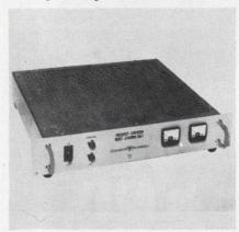
Series ATA frequency converters are stable sources of 400 Hz power operating from 50 to 70 Hz lines. Frequency stability, waveform purity and low dynamic impedance are reported. Output power is 100 to 1000 VA. Voltage regulation, from no load to full load, is 0.5%. Line regulation is  $\pm 0.5\%$ from 105 to 125 V.
