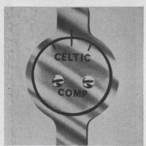
This miniature force ring switch can be installed in existing equipment with limited head space. Either compression or tension actuates contacts at specified loads to 1 ton. They have normally open or closed contacts and are capable of handling 5 A at 125 to 250 Vac. Accuracy and repeatibility of 1% and overload safety factor of 5 are claimed.
