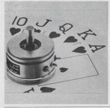
A single-turn pot meeting MIL-R-12934D is available in resistance ranges from 10  $\Omega$  to 100 k $\Omega$ . Tolerance is  $\pm 5\%$  from 10  $\Omega$  to 5 k $\Omega$  and  $\pm 3\%$  from 10 k $\Omega$  to 100 k $\Omega$ . Power rating is 2 W at 85°C. Gangable with up to 8 cups, it functions at 150°C. The 1-5/8-in. diameter pot is wirewound and offers a  $\pm 0.5\%$  independent linearity.
