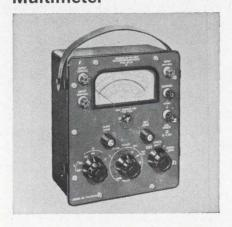
With more than 54 ranges, this solid-state multimeter covers dc and ac voltage and current, RF to 1.5 GHz and 2  $\Omega$  to 20 Megs center scale. Both Vac and dc have 11 ranges covering 12 mV to 1200 V full scale. Dc accuracy is  $\pm 2\%$  with 10 Meg/V input resistance. RF accuracy is  $\pm 0.5$  dB to 500 MHz. The meter is powered by 3D cell batteries.
