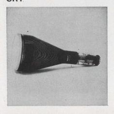
The D13-27 cathode ray tube has a 5-in. face and is 13.5-in. long. The tube features electrostatic focusing and deflection and has vertical sensitivity of 13 V/cm and horizontal sensitivity of 27 V/cm.
