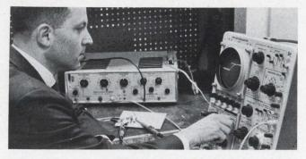
Tracing the key waveshapes. Circuit-designer Hilsenrath observes the step response of his common-emitter. By using a set of master response curves, he was able to predict performance before he built the network.
