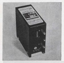
A modified dc-dc converter features fast switching rates, ability to function at 100° C, and rapid response to transient overvoltage. The "Thin-Verter" line has 24 to 30 Vdc input and 3 to 5000 Vdc output at 40 W. The model SHU converter measures 1-5/8- x 3-1/2- x 3-5/8 in. and weighs 26 ounces.
