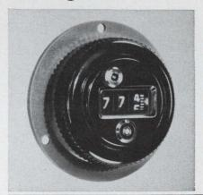
Flush or panel mounted, this rear-drive counting knob fits standard 1/4-in. shafts. One turn of the knob equals 100 counts. First figure wheel has 50 sub-divisions and the knob counts from 0 to 999.
