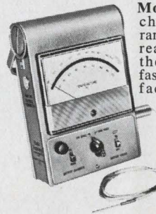
Model 380S —Direct-reading electrical thermometer measures liquid and surface temperature from -25 to +280^{\circ}\text{C} with one probe. Two ranges. Operates on series D flashlight batteries. $325. Complete with single crystal probe.
