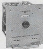
*P-122: 900 to 1300 MHz Sweep: 200 KHz to 400 MHz
