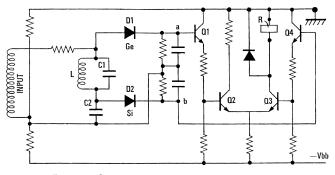
Figure 5 - Signaling receiver and discriminator circuit.
