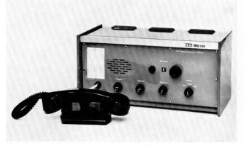
Marine very-high-frequency radiotelephone transceiver.
