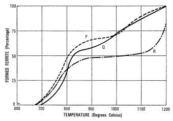
Figure 6 - Influence of manganese oxide on the kinetics of formation for mixed manganese-zinc ferrites.
