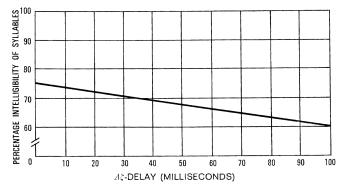
Figure 2 - Decrease in intelligibility with delay distortion (according to Lüschen, Küpfmüller). The reduction of intelligibility at point  $\Delta \tau = 0$  is caused by measuring equipment
