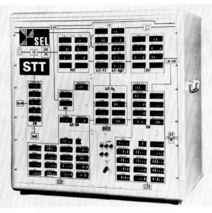
Figure 3 - Panel of memory for fault detection.
