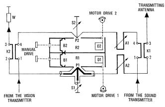
Figure 5 - Schematic of vision/sound combining unit.
