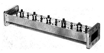
Figure 4 - Five-resonator direct-coupled waveguide filter.
