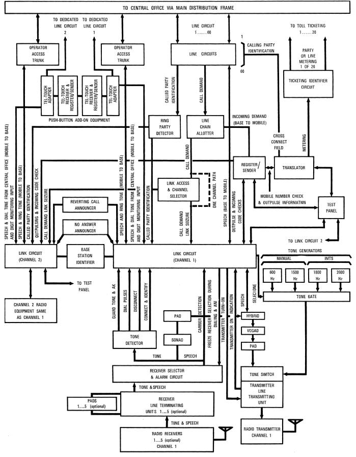
Figure 3 - Block diagram of base station. The Tel-Touch applique is in the upper left.
