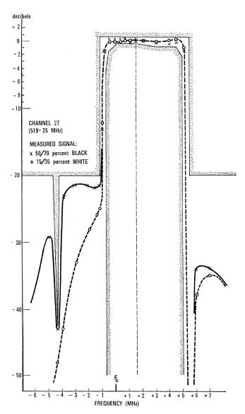
Figure 7 - Amplitude characteristic of sideband frequencies of a 10-kilowatt transmitter.
