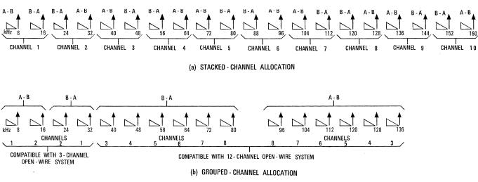
Figure 1 - Frequency allocation plans for stacked and grouped systems.
