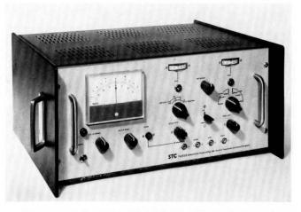
Test equipment for making differential measurements of phase and amplitude of color-television links.
