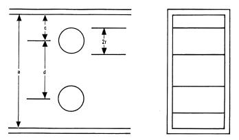
Figure 1 - Waveguide post doublets.
