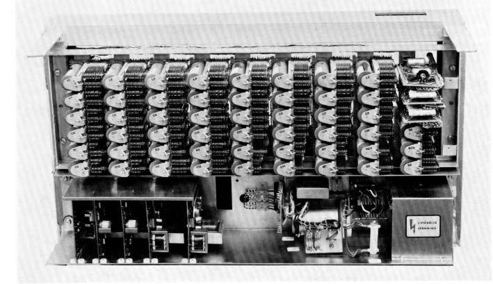
Figure 1 - A 16-line wall-mounted exchange with one cord circuit. Executive priority for one extension is included as a standard feature.
