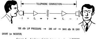
Figure 5 - Analogy of telephone circuit and SFERT.
