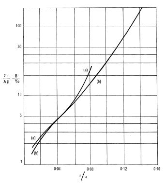
Figure 3 - Normalized susceptance of post doublets for  $\lambda_g = 2a$  and  $d = \frac{1}{2}a$ , (a) from Gruenberg's formula and (b) from (9).
