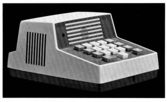
Figure 4 - Loudspeaking set. The keyboard is equipped with six special facility buttons.
