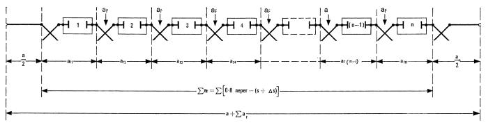
Figure 6 - 2-wire switching of a long-distance connection.
