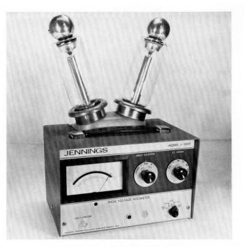
Portable instrument for measuring 100 kilovolts.
