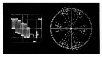
Figure 8 - Composite video with chrominance signal at the transmitter input.
