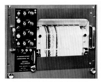
Paper recording using electrolytic marking for four channels.
