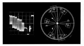
Figure 9 - Composite video with chrominance signal at the transmitter output.
