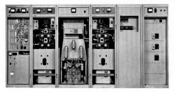
Figure 1 - Design of the 10/2-kilowatt television transmitter (from left to right):
