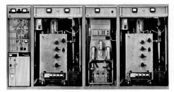
Figure 2 - The 40/8-kilowatt television transmitter (front row only from left to right):
