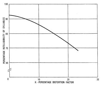
Figure 4 - Decrease of intelligibility with distortion factor k (according to K. Braun). The reduction of intelligibility at point k = 0 is caused by measuring equipment.
