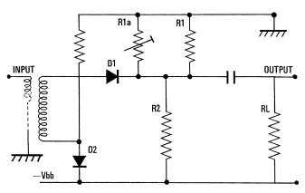
Figure 4 - Square-law detector with a suitably modified characteristic to reduce forward-voltage drop and maintain correct characteristic over working temperature range.
