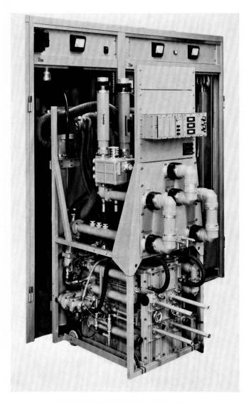
Figure 4 - 40/8-kilowatt combining unit.
