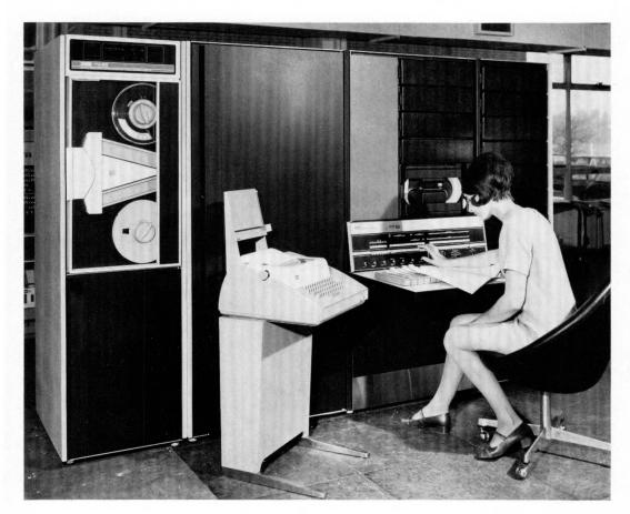
Control processor for *ADX* data switching equipment.
