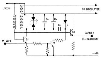
Figure 3 - Final oscillator circuit without biasing and matching details.
