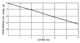
Figure 6 - Change in sound pressure level with altitude.
