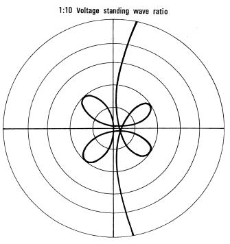
Figure 5 - Impedance plot for 5-resonator Chebyshev filter.
