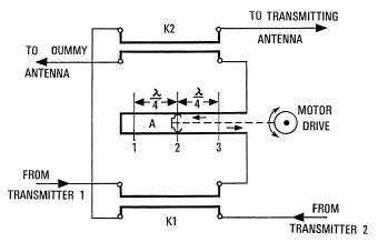
Figure 6 - Schematic of parallel transmitter operation.
