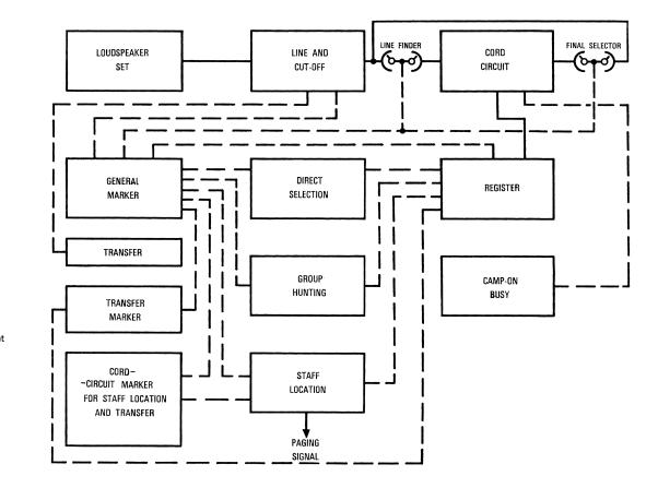
Figure 10 - Traffic lay-out 20-100 line exchange.
