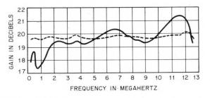
Figure 9—Gain-frequency characteristic over the trial route. The solid curve is before and the broken-line curve is after mop-up equalization, which limited the final spread to 0.55 decibel.
