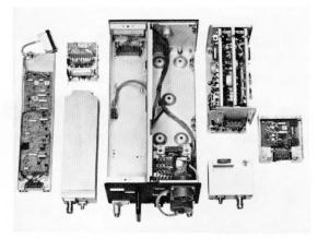
Figure 3—Modular construction of STR 70-P. From the left are the video unit, transmitter (front) and apparatus unit, chassis that has no active circuits but serves only for support and interconnecting, receiver (front) and power unit, and at extreme right the interface unit. The 3 units at the right are accommodated in the right half of the chassis unit.
