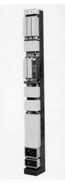
Figure 3—Front view of the slimrack. At the top is the alarm indicator while the 3 panels immediately below are the squelch, end amplifier, and distribution amplifier. The pre-amplifier is next and beneath it are the equalizer, intermediate-frequency amplifier, and meter panel. The next three units are the receive local oscillator, power amplifier, and transmit local oscillator. At the bottom are the transmit and receive power units.
