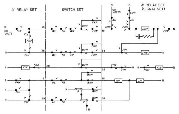
Figure 5-Signal control for geographic system.
