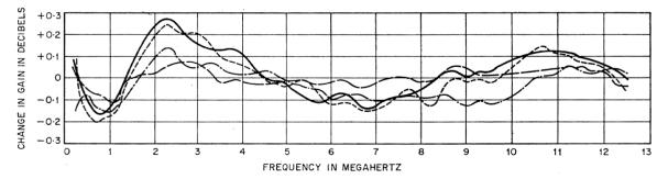
Figure 15—Variations of gain of the trial installation relative to values measured on 7 April 1966 with a cable temperature of 5.5 degrees Celsius.
