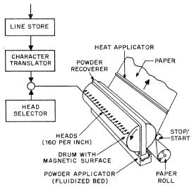
Figure 14—Arrangement of Ferrodot high-speed printer.
