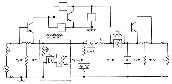
Figure 1-Line amplifier circuit.
