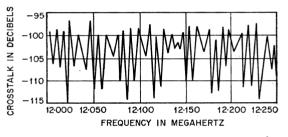
Figure 14—Crosstalk measured at close frequency intervals for the trial installation.
