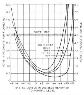
Figure 10—Performance of the trial route when loaded with white noise. The limit of 3 picowatts per kilometre (4.8 picowatts per mile) set by the International Telegraph and Telephone Consultative Committee (CCITT) is indicated.
