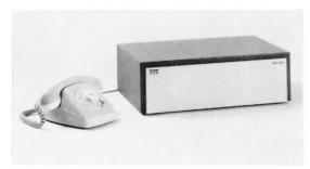
Figure 19—Modem equipment *GH-1101* housed in a desk-top cabinet.
