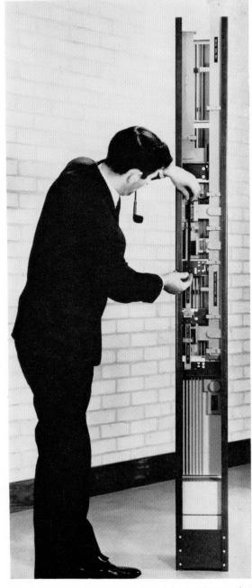
Figure 2—Rear view of the slimrack showing vertical waveguide runs.
