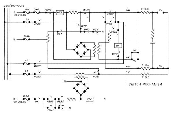
Figure 1—Switching machine is operated from 3-phase power supply.
