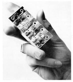
Figure 11—A television tuner using voltage-adjustable diode capacitors in *DO-7* glass mounts. The diodes may be seen in the centers of the three middle sections.
