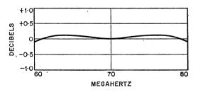
Figure 8—Transmitter-to-receiver response-frequency characteristic for an input level of -65 decibels referred to 1 milliwatt corresponding to a 35-decibel fade.
