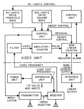
Figure 1—General division of functions in STR 70-P altimeter.
