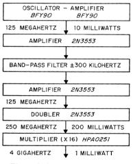
Figure 5-Receive local oscillator.
