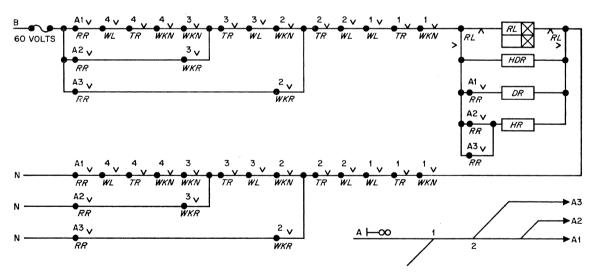
Figure 2-Signal control circuits with relay interlocking.
