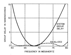
Figure 9—Group delay for a single hop at a superhigh-frequency nominal input of -30 decibels referred to 1 milliwatt.
