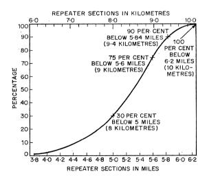
Figure 4—Percentage of repeater sections below the stated lengths for 30 routes of 4-megahertz 960-channel systems.
