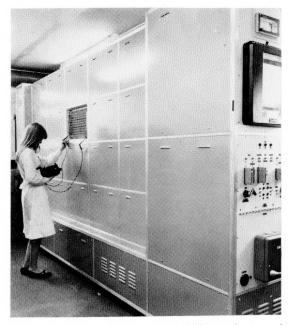
Figure 1—Life test rack on which 2557 transistors and 4743 diodes were burnt-in for three months, without any failures. The rack applies the submarine repeater operation conditions with an elevated device case temperature.
