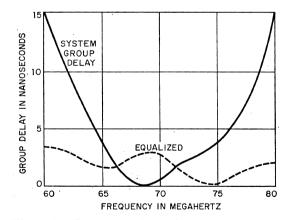
Figure 10—Group delay for a single hop at a superhigh-frequency input of -65 decibels referred to 1 milliwatt corresponding to a 35-decibel fade.
