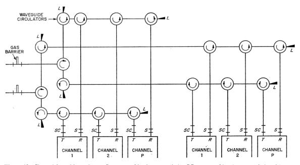
Figure 12—Channel branching scheme. S = waveguide shutter switch. SC = waveguide shutter switch with test point on transmitter side. L = waveguide load. T and R are transmit and receive halves of the indicated channels.
