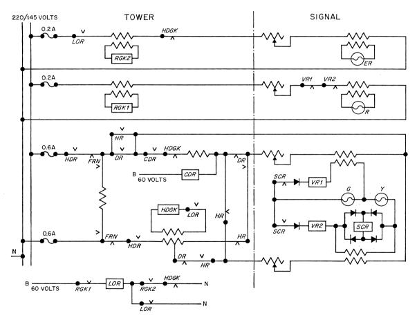
Figure 6—Light signal circuits.
