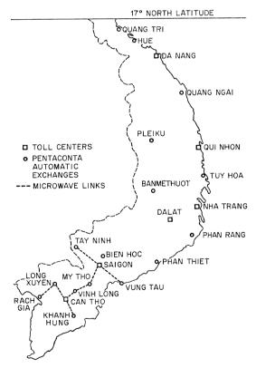
Figure 8—Installations in South Vietnamese nationwide telecommunication system.
