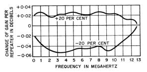
Figure 13—Variation of gain per amplifier with changes of 20 per cent in power-feeding currents.
