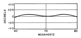
Figure 7—Transmitter-to-receiver response-frequency characteristic for a nominal input level of -30 decibels referred to 1 milliwatt.
