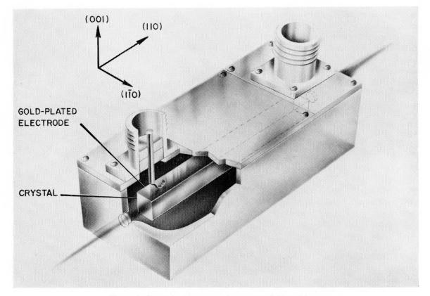
Figure 4—Internal arrangement of transverse-field modulator.
