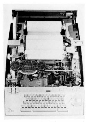
Figure 2-Teleprinter with silencing cover removed.
