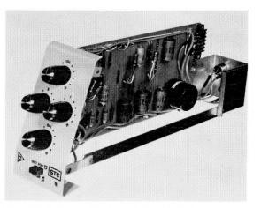
Figure 12—A microphone amplifier built into a singlewidth module unit. The method of construction combines adequate rigidity with ease of access for servicing.
