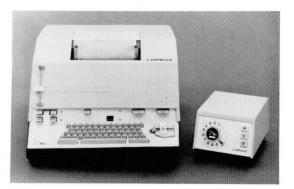
Figure 10-Teleprinter with separate subscriber box.
