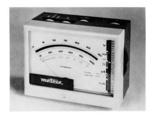
Figure 11—Millivoltmeter VX 203 A with selector control visible.
