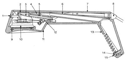
Figure 3-Sectional view of the handset.
