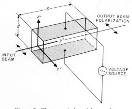
Figure 2—Electro-optical modulator using transverse field.
