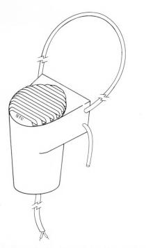
Figure 6—Type 4124 miniature lavalier moving-coil microphone.
