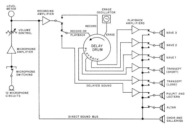
Figure 17-Layout of magnetic-drum delay unit.
