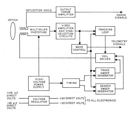
Figure 2—Block diagram of fine-guidance sensor.
