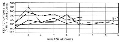
Figure 7—Arithmetic mean values of the key actuation times. Curves A and B were measured in 1964; they represent 7259 and 3188 key depressions, respectively. Curves C and D were measured in 1965 and represent 13 670 and 7259 key depressions.
