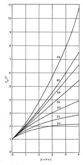
Figure 6—Transition frequency ratio versus class over lapping for values of X indicated on the curves. F= transition frequency,  $F_0$  = transition frequency for n = 0 (disjoint classes), N = 100, a = 84.06 erlangs, B = 0.01, and h = 180 seconds.
