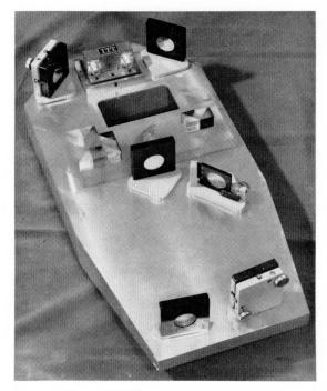
Figure 15-Electro-optical front end.
