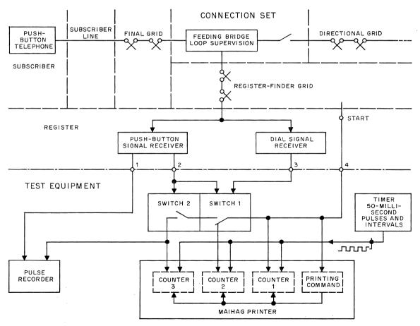
Figure 2-Block diagram of the test setup.
