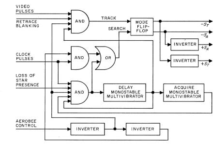
Figure 4—Block diagram of mode control circuits.
