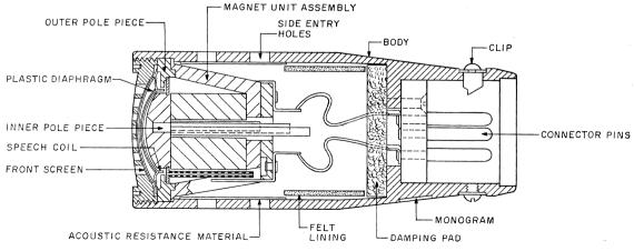
Figure 1.—Type 4105 unidirectional moving-coil microphone.
