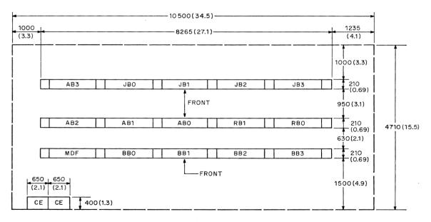
Figure 1—Floor plan for 1000-line exchange with 72 trunks and 64 local connecting circuits using fixed frames 2.81 meters (9.2 feet) high and weighing approximately 450 kilograms per running meter (300 pounds per running foot). Dimensions are in millimeters (feet). The functions of the frames are as follows:
