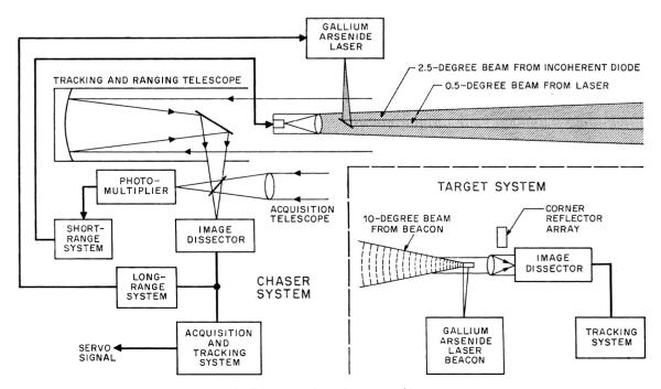
Figure 12-Diagram of rendezvous guidance system.
