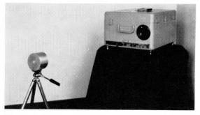
Figure 7—Breadboard arrangement for electro-optical direction and ranging system (EODAR).
