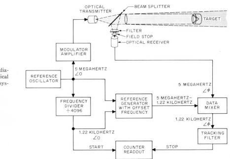
Figure 8—Simplified diagram of electro-optical direction and ranging system (EODAR).
