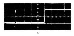
Figure 3—Pulse and bar response. A is the input, B the output of the encoder drive amplifier working into a resistive load, and C is the final output. The horizontal scale is 2 microseconds per division.
