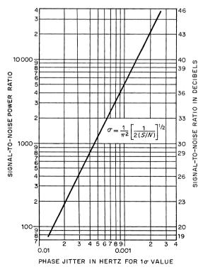
Figure 9-Phase jitter versus signal-to-noise ratio.
