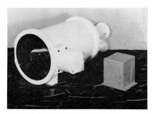
Figure 11—Prototype optical rendezvous guidance system.
