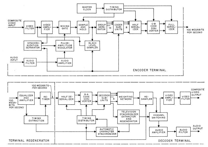
Figure 1-Schematic diagram of 81-level pulse-code-modulation system.
