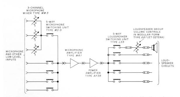
Figure 13-Diagram of a sound system engineered from standard elements of the modular public-address equipment.
