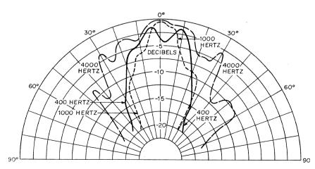
Figure 11-Polar response characteristics of column loudspeaker.
