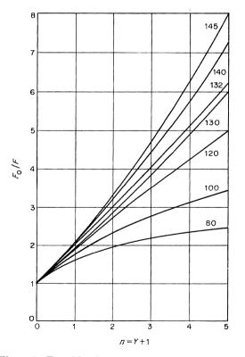
Figure 5—Transition frequency ratio versus class overlapping for values of X indicated on the curves. F = transition frequency,  $F_0$  = transition frequency for n = 0 (disjoint classes), N = 150, a = 131.58 erlangs, B = 0.01, and h = 180 seconds.
