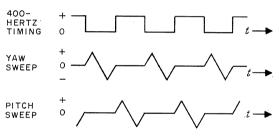
Figure 6-Track scan waveforms.
