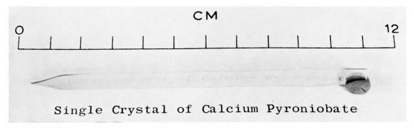
Fig. 17—A ribbon crystal of calcium pyroniobate. The reflections of the caption seen in the (100) mirror facets are precisely doubled owing to extreme parallelism of opposite sides of the ribbon.
