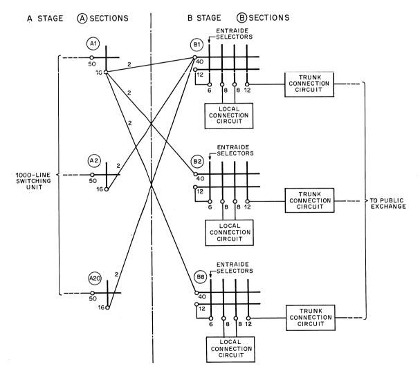
Figure 2-Link arrangement for 1000-line switching units.
