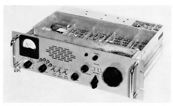
Figure 9-Rack version of TransITT very-high-frequency marine radiotelephone set showing Ministac construction.
