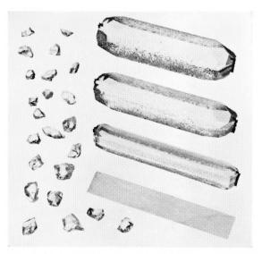
Figure 4—Natural quartz chips (left) provide the material that crystallizes from solution onto seed plates (as bottom right) to give large blocks of synthetic quartz (right). Crystals grown for manufacture of different sizes of resonator blanks are shown. Block length approximately 22 centimetres (8.8 inches).
