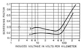
Figure 10—Production-control screening-factor curves at  $16\frac{2}{3}$  hertz. A = 1.2-millimeter 12-quad cable with 1.0-millimeter aluminum sheath. B = 1.2-millimeter 4quad cable with 0.9-millimeter aluminum sheath. Refer to Table 4.
