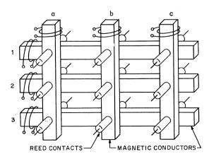
Figure 2—Crosspoint matrix with simple linear addition of the actuating energy distributed to two coordinate directions.
