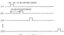
Figure 6-Clock pulses.
