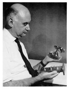
Figure 16—George Craven, the inventor, shows how a 3-section, 4-gigahertz filter of the new evanescentmode type compares with a conventional filter, the volume of which is 8 times greater. The new filter is built in X-band waveguide with a cross section of 0.9 by 0.4 inch (2.3 by 1 centimeter).
