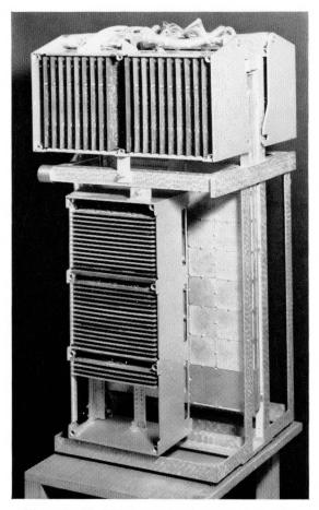
Figure 7—Model 3 memory with access electronics.
