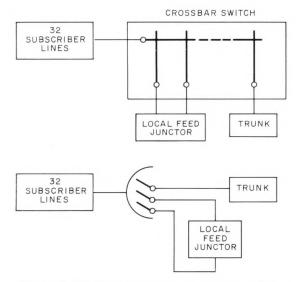
Figure 2-Single-stage version of primary switch.
