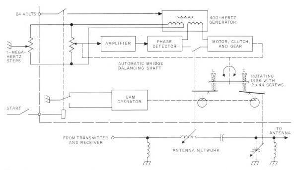
Figure 3—Antenna tuning unit. Adjustment for each of 44 steps of 1-megahertz each is by 2 screws that control the adjustable inductor and capacitor in the antenna network. The cams push the arms away from these setscrews and close the switch to the motor when the disk is to be rotated for a new channel.
