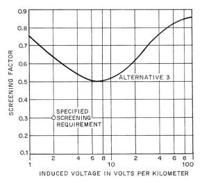
Figure 5-Measured screening-factor curve of alternative 3 for 1.2-millimeter 27-quad cable at 16<sup>2</sup>/<sub>3</sub> hertz.
