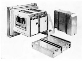
Figure 6-Transmitter-receiver, interior view.
