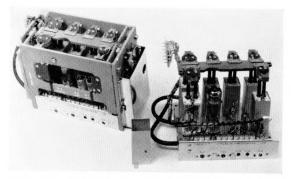
Figure 7—At left is the complete transmitter tuning stage, while at right is a partly disassembled unit.
