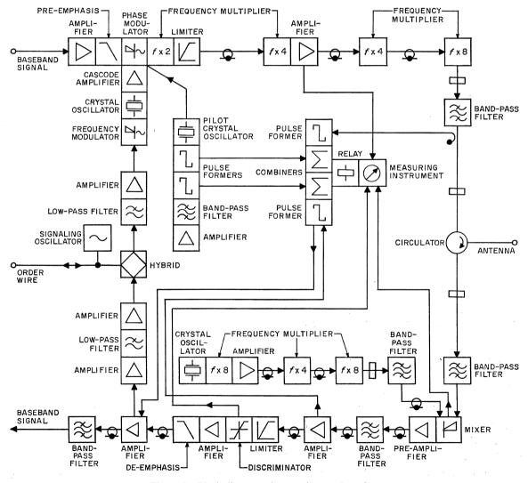
Figure 2-Block diagram of transmitter and receiver.
