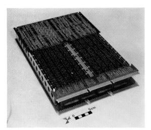
Figure 9—Matrix consisting of crosspoint strips of the type shown in Figure 8.
