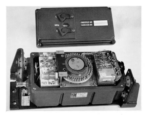
Figure 11—Automatic antenna tuning unit, cover removed.
