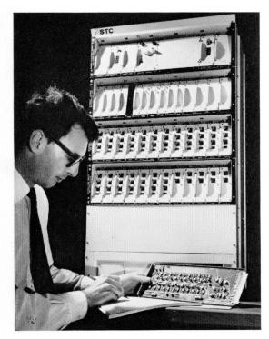
Figure 9—Pulse-code-modulation terminal equipment for a 24-channel public telephone system.
