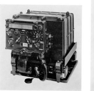
Figure 4—Transmitter-receiver with control unit attached.
