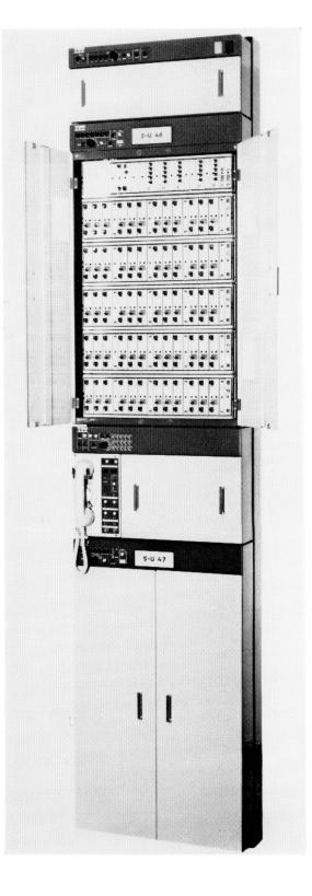
**Mobile Television Transmitter for Temporary Service**—A complete television transmitter has been built in mobile form for use during major overhaul or other construction work in a permanent installation.
