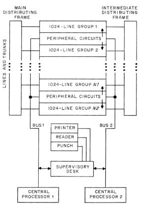
Figure 1—Modular network and central control of 10-CX system.
