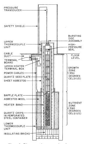
Figure 2—Diagrammatic cross-section of quartzgrowing installation.
