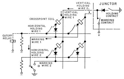
Figure 4—Marking procedure in a crosspoint matrix.
