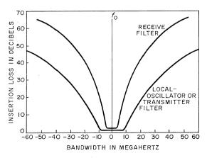
Figure 3—Insertion loss of waveguide filters as a function of bandwidth.
