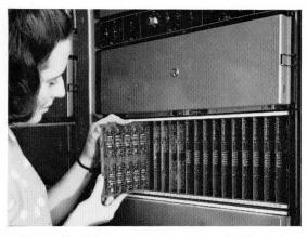
Figure 19—All parts are mounted on plug-in cards, and Minibell type paraplate modules are used.
