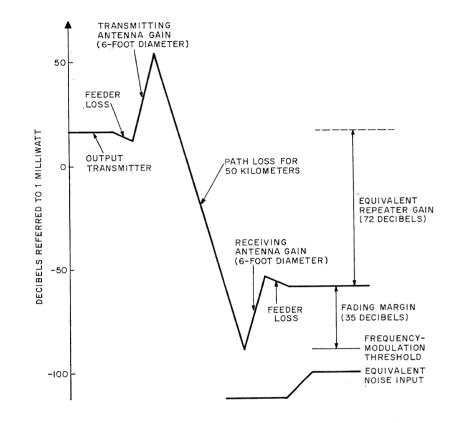
Figure 1 — Performance characteristics for an intermediate-frequency bandwidth  $B_{1t} = 1.5$  megahertz and a noise figure of 12 decibels. The equivalent noise input =  $KTB_{1t}$ .
