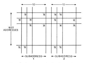
Figure 7—Capacitor matrix. The absence of a capacitor at a crosspoint gives a  $\theta$  output.
