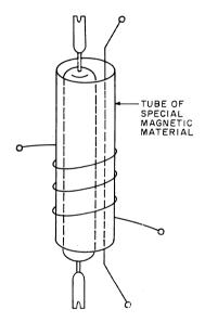
Figure 4—Crosspoint element using a tube of magnetic material having two directions of easy magnetization.
