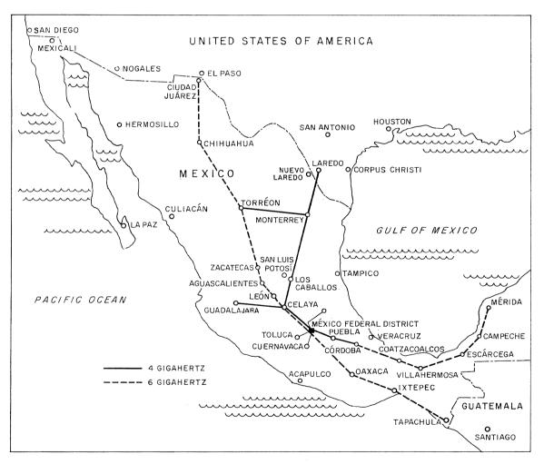
Figure 4—The original 960-channel 4-gigahertz radio network for Mexico will be extended with 1800-channel 6-gigahertz equipment as shown.
