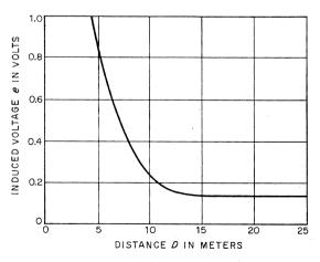
Figure 1—Induced voltage e per 100 ampere-kilometers as a function of distance D from middle of track (experimental results from southwest Norway on a stretch with booster transformers).
