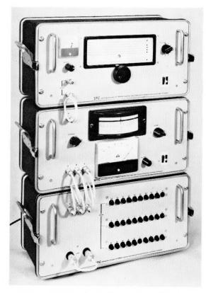
Figure 13—Insertion-loss measuring equipment type 74905.
