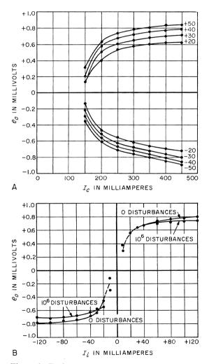
Figure 3—Typical output characteristics of the memory cell. A shows  $e_o$  as a function of  $I_o$  for the indicated values of  $I_i$  in milliamperes. B shows  $e_o$  as a function of  $I_i$  for  $I_o = 250$  milliamperes.
