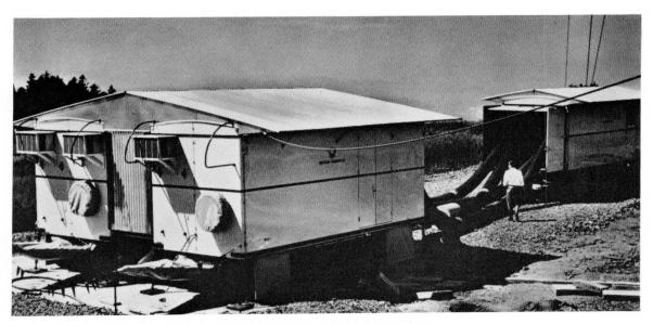
Figure 3-Mobile television transmitter.
