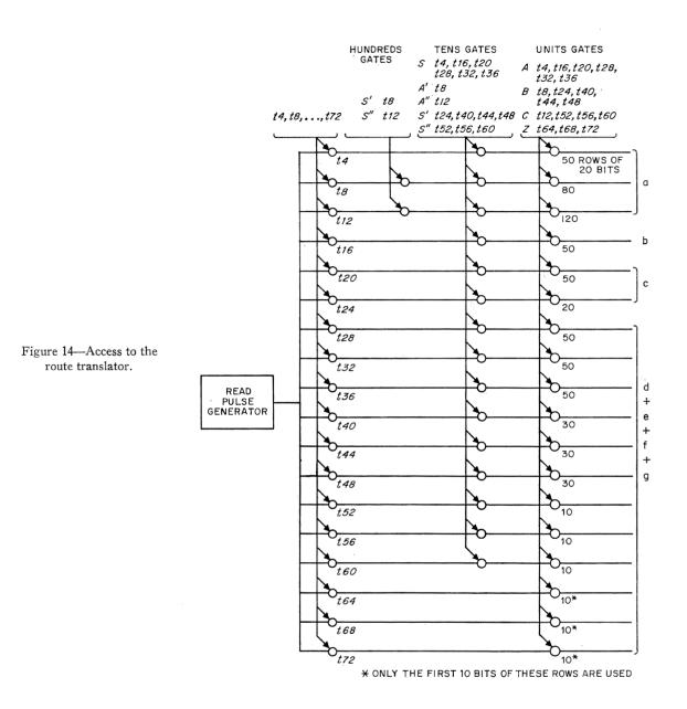
interval t8. All 20 bits of this row are interrogated but only the first 10 are sent to recorder 3, where the answer is made available. As indicated, the 10 figures A' are rearranged into 5 groups of 2 for driving the five T gates and in 2 groups of 5 for driving gates C1 and C2, respectively.
