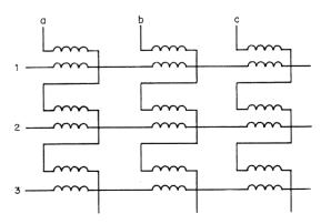
Figure 3—Crosspoint matrix using linear addition of electromagnetic energy distributed to two coordinate directions.
