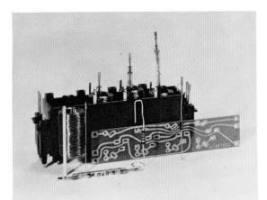
Figure 6—Standard building block containing 4 reed crosspoints.
