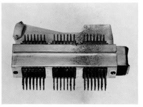
Figure 8-Plugs and jacks, separate and engaged.
