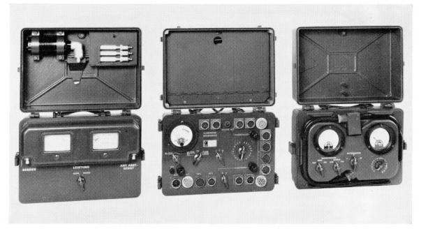
Figure 15-Test equipment. From left to right are the reflectometer, cable tester, and communication-set tester.
