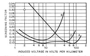
Figure 6—Measured screening-factor curves on handmade samples of 1.2-millimeter 27-quad cable at 16<sup>2</sup>/<sub>3</sub> hertz. Refer to Section 3.2.
