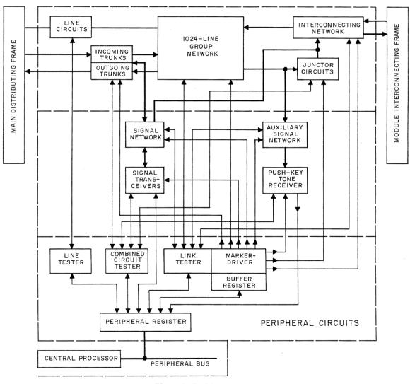
Figure 2—Peripheral package.
