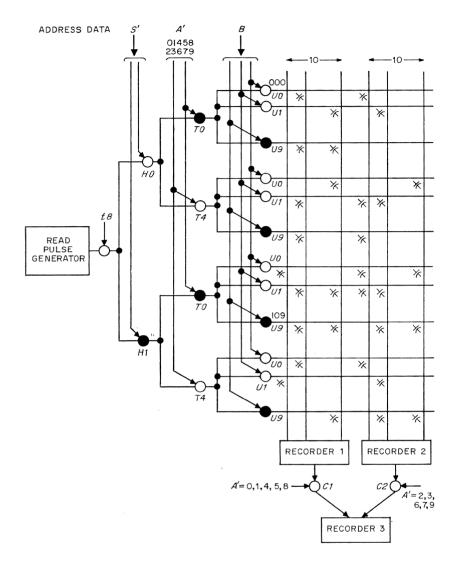
Figure 13—Principle of access gating for 160 S'A'B combinations of the number-of-digits section.
