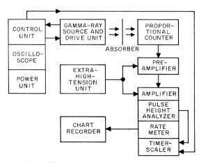
Figure 15—Arrangement of components in the Mössbauer spectrometer.
