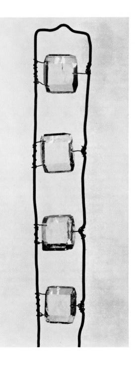
Figure 1—First crystals produced during project. These are approximately 2 centimetres square and 7.5 millimetres thick.
