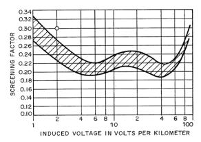
Figure 8—Production-control screening-factor curves for 1.2-millimeter 19-quad cables at 16<sup>2</sup>/<sub>3</sub> hertz (1.1millimeter aluminum sheath). Normal variations (gap approximately 45 percent). Refer to Table 4.
