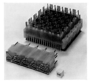
Figure 10—Crosspoint strip holding 4 crosspoint elements, each with 3 type H 50 reed contacts for continuous hold current. The crosspoint matrix shown consists of 4 crosspoint strips with 4 crosspoint elements each.
