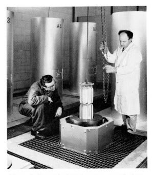
Figure 5—Removal of newly grown crystals from autoclave.
