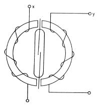
Figure 5—Principal structure of the ferreed.
