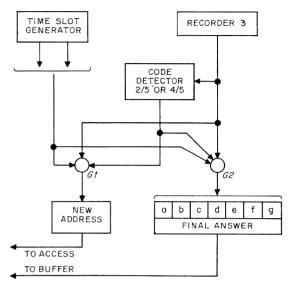
Figure 16-Transcoding and display.
