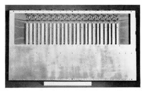
Figure 6-Memory matrix of model 3 during assembly.
