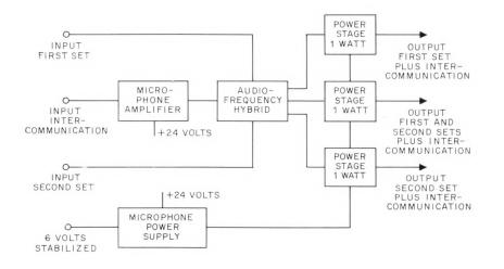
Figure 12—Intercommunication-amplifier arrangement.
