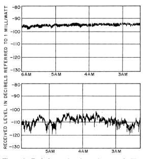
Figure 9—Typical recorder charts for path 2. The upper chart was made on 3 October and the lower chart on 1 October 1962.
