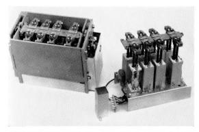
Figure 8—The receiver tuning stage is at left, and the partly disassembled receiver chassis is at right.
