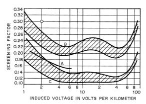
Figure 11—Curve A is the effective screening factor between Å1 and Ustaoset. B and C are the factory measured screening-factor curves for 19-quad and 27-quad cables, respectively.
