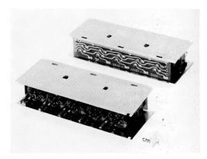
Figure 8—Crosspoint strip holding 5 crosspoint elements, each with 4 type *H* 50 reed contacts for continuous hold current.
