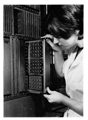
Figure 7—Plug-in line switch unit containing 6 sets of 4-by-4 crosspoint matrices.
