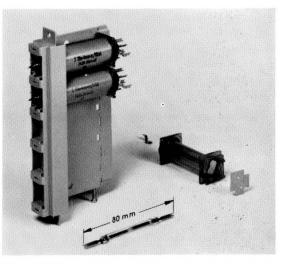
Figure 7—The coil form at the right holds 2 of the 80-millimeter (3.1-inch) reed-contact elements. A crosspoint strip to hold 5 complete reed switches is also shown.
