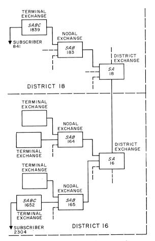
Figure 1-Star-shaped telephone network.
