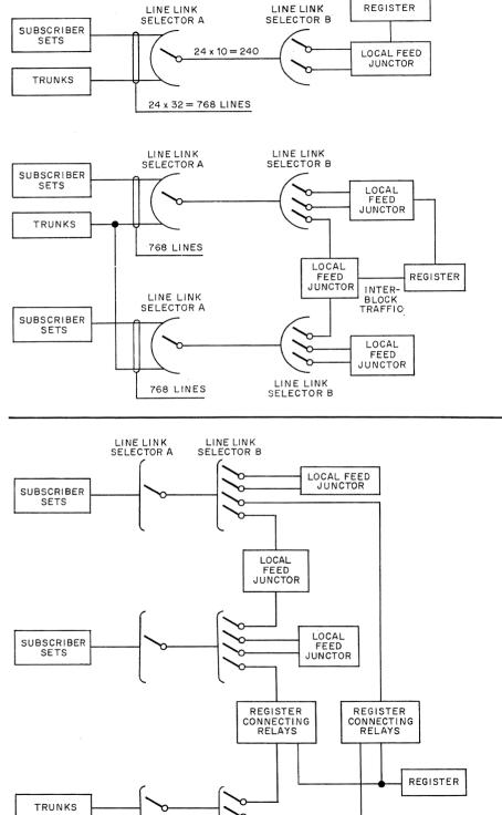
Figure 4—Two-stage version of primary switch. At top is the single-block exchange with a maximum of 768 terminals. Below it is a 2-block exchange.
