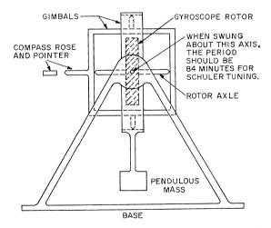
Figure 3—Schuler tuning employs a pendulum having a period of 84 minutes that when moved from its vertical position causes an oscillation about the indicated axis. The error does not continue to increase with time but oscillates back and forth at the Schuler period.
