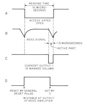
Figure 12-Read cycle of capacitor store.
