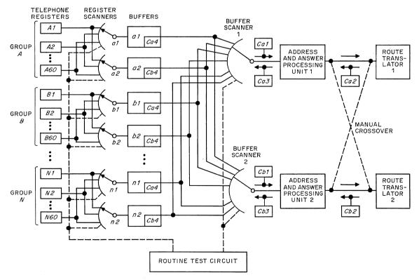
Figure 18-Block diagram of number analyzer.
