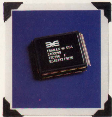
1991-TEC256. The first Fast and Wide SCSI disk controller also boasts the fastest disk data rate and highest system bandwidth.
