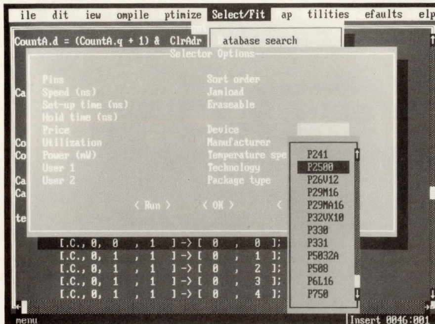
Using a library of 6000 devices representing 300 architectures, SmartPart offers a range of criteria for optimal device selection.
