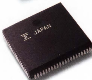
1.5 \mu 3000 Gate CMOS Gate Array
