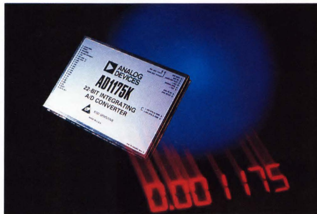
With its 133-dB dynamic range, ±1-ppm maximum integral nonlinearity, and modular package, Analog Devices' AD1175 competes with 6.5-digit DVMs.
