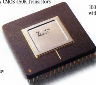
32-bit IEEE Floating-Point General Purpose DSP 1.2 \mu CMOS 450K Transistors
