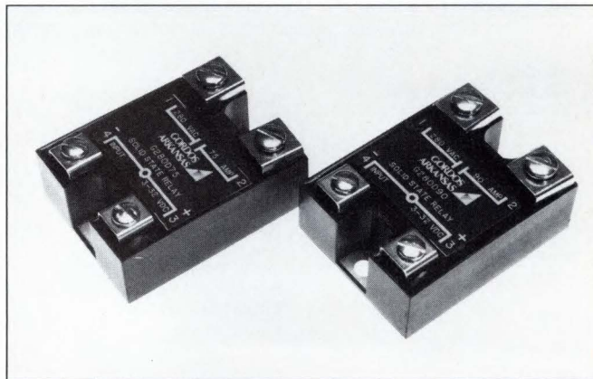
Offering load ratings to 90A at 480V ac, G Series solid-state relays from Gordos employ dual back-to-back SCRs for output switches and feature 4000V rms optical-type input-to-output isolation.
