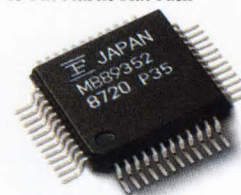
SCSI Protocol Controller with On-Chip Drivers, 48 Pin Plastic Flat Pack
