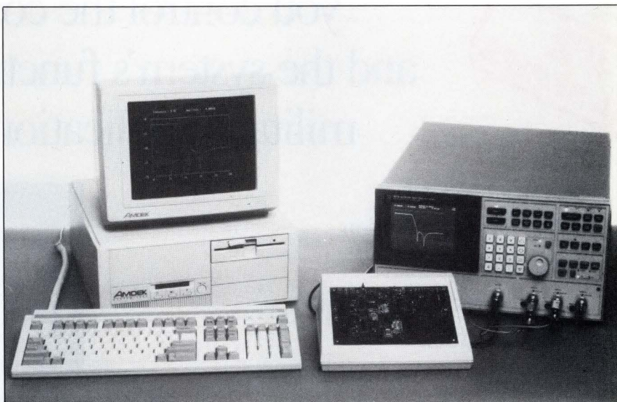
The design kit for the SC22324 programmable filter includes software, a textbook, and a programming station that connects to an IBM PC.
