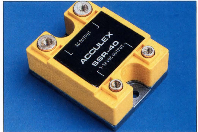
To virtually eliminate EMI/RFI problems, SSR Series solid-state relays from Acculex employ zero-sense circuitry that provides long-life zero-voltage turn-on and safe zero-current turn-off.
