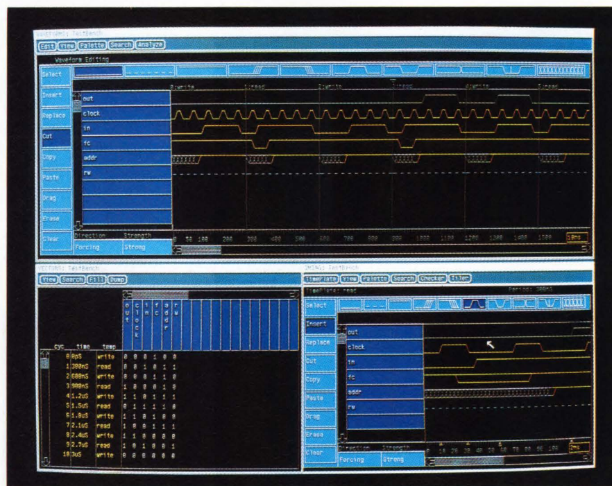
A behavioral data-management system that lets you interactively create signal definitions, device timing, data patterns, and waveform displays (Test Systems Strategies Inc)
