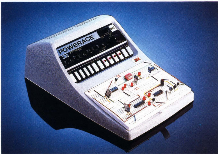
A solderless breadboard with power supplies, logic switches, and removable circuit boards (3M)
