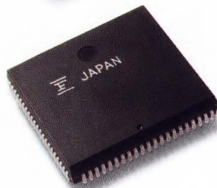
1.5 \mu 3000 Gate CMOS Gate Array
