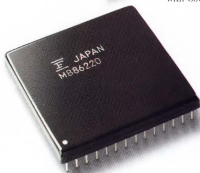
24-bit Floating-Point General Purpose DSP 1.2 \mu CMOS 135-PGA
