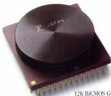
12K BiCMOS Gate Array with Cooling Tower
