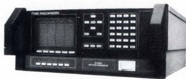
Pulse Instruments PI-6500 Pattern Generator.
