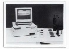
identify individual wafers for process control. The system includes a 68000-based single-board computer in a chassis, a video monitor, a trackball for operator input, menudriven software, and as many as eight cameras. 8-station system, approximately \$66,000.
