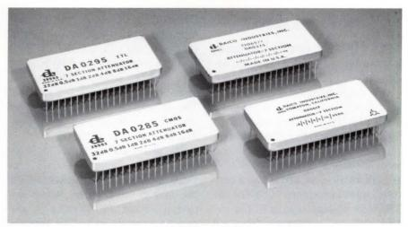
**To accommodate high frequency and power needs,** Daico Industries offers a line of 7-bit attenuators that operate over the 30- to 500-MHz range and accept input power levels of 13 dBm. They operate from a 5V supply.
