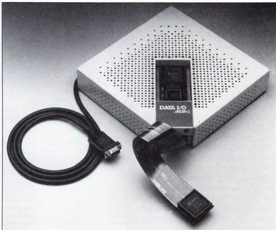
More than just an in-circuit emulator, the Mesa I combines modeling, emulation, simulation, and analysis functions to use with programmable gate arrays.
