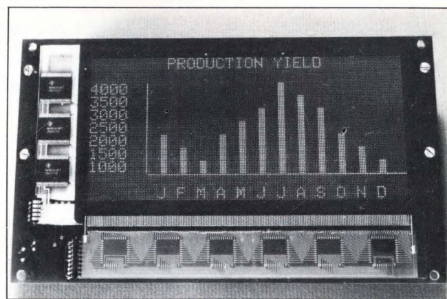
If your application involves message-and graphics-type displays, you'll want to evaluate the APD-192G088-1 plasma panel from Dale. The self-contained unit includes a 192-column \times 88-row display window, drive electronics, and a \mu\text{P} -based controller.
