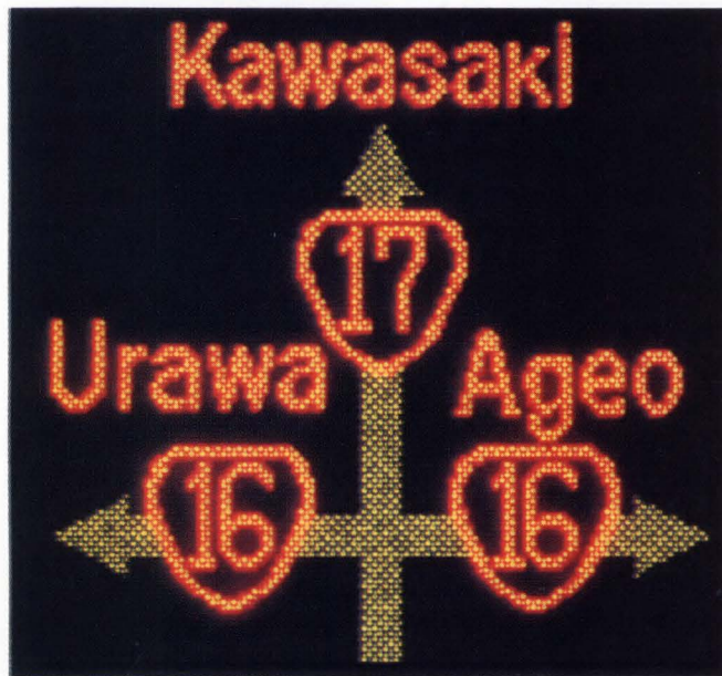
Particularly well suited for outdoor applications, the LT144M display module from Sharp uses a 16 \times 16 grid of dichromatic LEDs. Onboard electronics allows you to use multiple modules to create displays containing a combination of graphics and characters.
