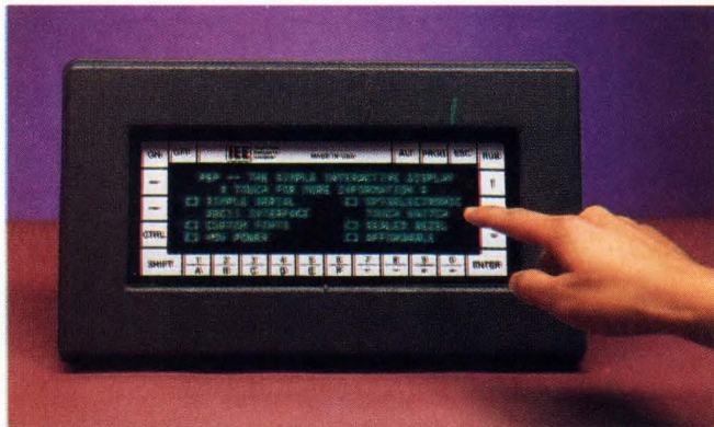
Combining a 6-line \times 40-character VF display with an infrared touchscreen, IEE's 4283-01 display module features 969 switch (touch) locations and is immune to false triggering by ambient light.
