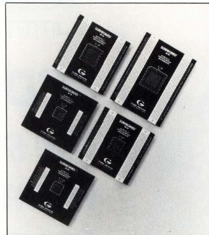
Development tools with a twist are these adapters from Global. They socket a surface-mount package and let you make connections to the part by using solderless breadboarding strips.
