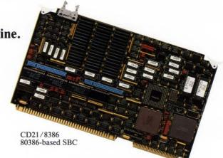
• We provide a socket for the 80387 numeric data processor and the Weitek WTL1167 floating point co-processor board. Intel supports only the 80387.
