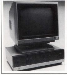
encrypted and nonencrypted modes. In its encrypted mode, the transceiver transmits at either 2400 or 4800 bps, depending on the type of STU-III voice/data telephone-encryption terminal you use. In its nonencrypted mode, the transceiver operates over standard telephone lines at 9600 bps. The transceiver accepts input from a wide variety of still and motion video
