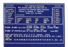
InSight Display. InSight blends analyzeremulator techniques to give you continuous, real time monitoring of key processor functions. And still services user interrupts. It displays changing register contents, I/O lines, ports, user-defined memory windows. With your own labels.
