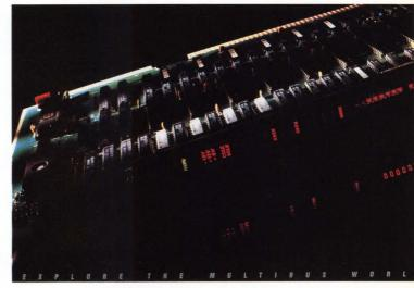
**Board-based bus analyzers** give you a simple, convenient window for observing minicomputer or microcomputer bus operations. (Photo courtesy Silicon Control Inc)
