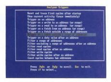
**Analyzer Triggers.** Commonly used triggers can be selected quickly from a list of standard and user-defined triggers.
