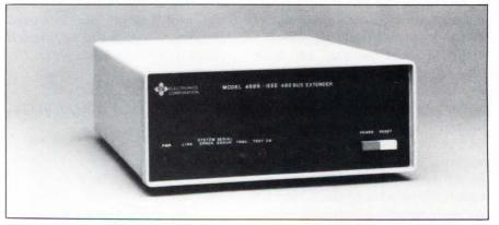
Maintaining a 300k-byte/sec data transfer rate, the IEEE-488 bus extender handles distances as great as 500m using coaxial cable or 2000m using fiber-optic cable.
