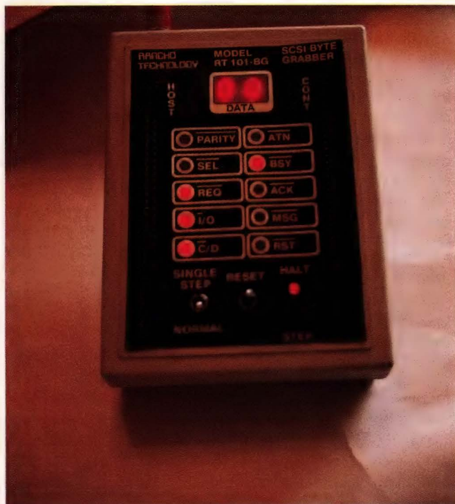
Single-stepping through SCSI bus operations is possible with the Rancho Technology SCSI Byte Grabber. This capability allows you to inexpensively debug SCSI firmware.
