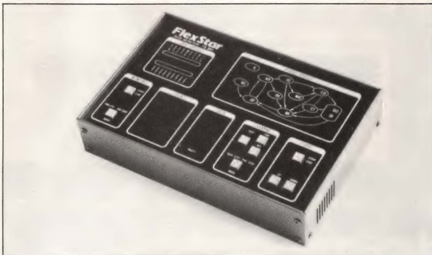
An 8k-byte buffer captures SCSI bus activity in the Flexstar bus monitor. The product includes a parallel-printer port, so that you can subsequently print the data.
