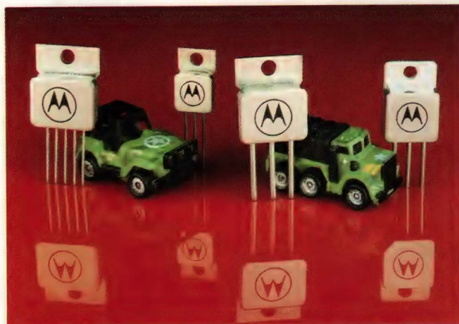
These hermetic packages from Motorola resemble the plastic TO-220 and TO-247. These housings let you replace the old, bulky TO-3 in environments requiring hermeticity.
