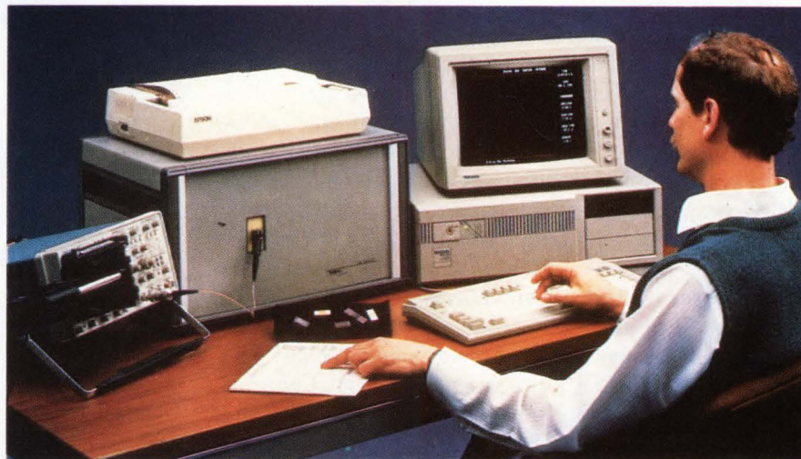
System characterizes components according to the latest MIL-STD-883 requirements (Trisys Inc)
