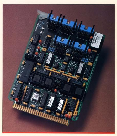
The ZT 88CT41 Quad Serial Interface is one of several Ziatech CMOS boards with low power consumption and a wide temperature option for harsh environments. This I/O board provides additional RS-232-C and/or RS-422-A/485 channels to STD Bus systems.
