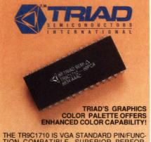
THE TR9C1710 IS VGA STANDARD PIN/FUNCTION COMPATIBLE. SUPERIOR PERFORMANCE: INTEGRATED COLOR LOOK-UP TABLE, TRIPLE VIDEO DAC, LOGIC & ANALOG INTERFACE ON 1 CHIP REDUCES SYSTEM COST. ENHANCED (256) COLORS. UNLIMITED ACCESS TO LOOK-UP TABLE. 66 MHZ CLOCK RATE. FOR A BETTER SYSTEM SOLUTION, CALL 800-288-1874.
