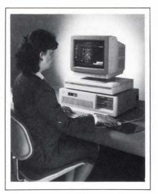
and has text handling capabilities as well. The package includes CADRE-II design/drafting software and a coprocessor module. The module contains a Motorola 68020 32-bit µP, used as a coprocessor, and 4M bits of RAM, loaded with the Cadra-II software on bootup. An AMD 29116 16-bit µP running alongside a custom gate array power the graphics.
