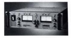
trol the output with an external ±10V source. An optional digital control board allows you to program most of the unit's functions via the IEEE-488 bus or an RS-232C datatransfer bus.
