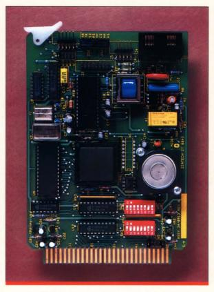
The ZT 8843 is a 300/1200/2400 BAUD Modem for STD Bus computers, compatible with industry standard Hayes<sup>TM</sup> AT Command Set.
