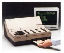
electronics stores device-specific instructions on a 3½" micro diskette. To update your UniSite 40 with the latest device releases, simply load a new master diskette.
