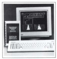
visual or symbolic data manipulation, and allows you to work with fuzzy logic. The package includes sample neural networks, including some that perform optical-character recognition, speech synthesis, image recognition, and image enhancement. To run the program, you need an IBM PC or compatible that has at least 256k bytes of main memory and runs under DOS 3.0 or higher. \$99.95.
