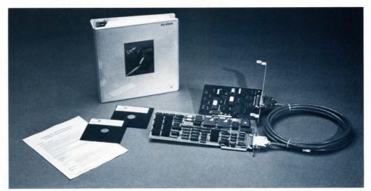
This evaluation system includes the XL-8200-40 raster-printer-controller board, the printer-interface module, Weitek's Postscript-compatible interpreter, and documentation. It's priced at \$15,000.
