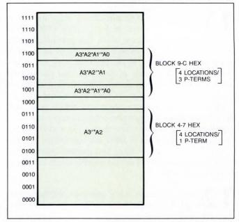
Fig 5—Product-term consumption varies with block size and base address.
