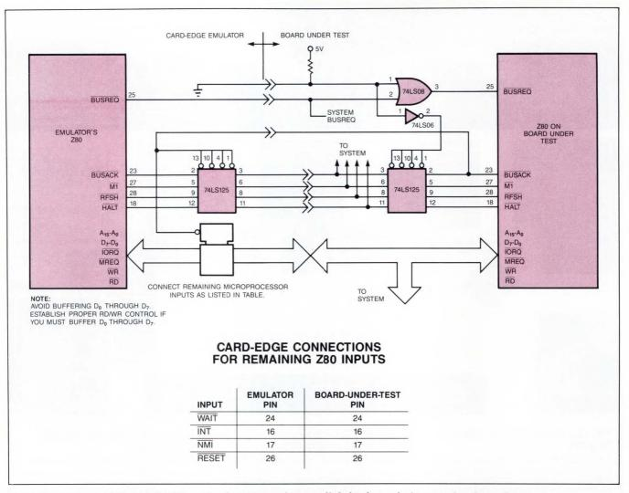
Fig 5—Card-edge emulation for the Z80, as for the 8086, requires very little hardware that's external to the emulator.
