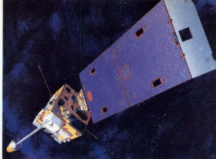
The National Oceanic and Atmospheric Administration's Geostationary Operational Environmental Satellites (GOES), under construction by Ford Aerospace & Communications Corporation, will provide improved capabilities for weather forecasting. GOES will have a microprocessor-based altitude-control system.
