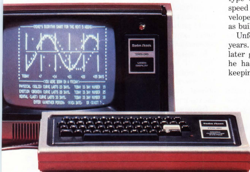
The original TRS-80 microcomputer was unveiled in August 1977. The system cost $399 and offered a basic 4k bytes of memory, a Z80 processor, Basic, and cassette tape storage.
