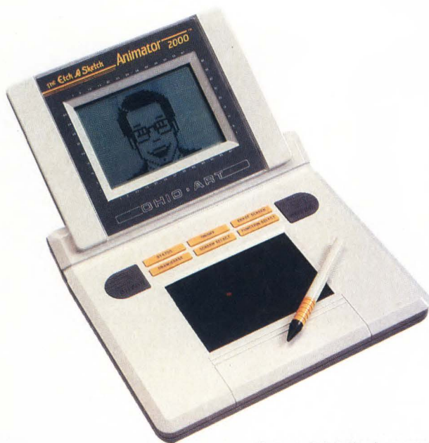
Electronic Etch A Sketch, powered by a Hitachi 6301 microcontroller, allows young (and young-at-heart) artists to create animation sequences.
