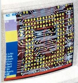
he Integrated PADS-Superstation is a new and powerful PC-Based Design Station that allows the Engineer or Circuit Designer to perform the entire design sequence from cradle-to-grave. Every decision required in the design effort, from Logic Capture to Printed Circuit Design, to 100% Connection Routing, to Checking, to generating Manufacturing Aids is made by the responsible engineer and implemented on a single, fully integrated CAE/CAD SUPERSTATION!
