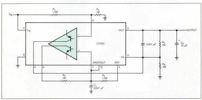
Fig 1—This battery-powered regulator circuit shuts itself down when the battery is depleted and doesn't resume supplying power until the battery is recharged.
