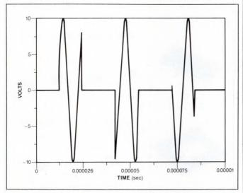
Fig 3—Using the intervals specified for  $V_P$  in Listing 1 to gate a sine wave on and off produces this waveform.
