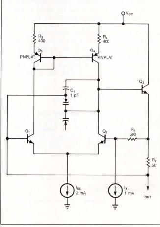
Fig 16—This almost-all-npn current source has a wide compliance range: from about 2V below  $V_{CC}$  down to the breakdown voltage of the npn devices.
