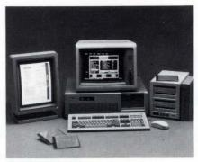
CAPS is a PC-based hardware and software package that utilizes a high-resolution monitor and a 4-disk CD-ROM player to automate the time-consuming process of selecting ICs and semiconductor devices.
