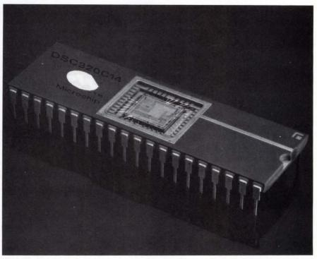
ROM, RAM, timers, and digital I/O signals combine with a DSP320C10 µP core in the DSC320C14 DSP microcontroller. The chip fits into real-time control applications that benefit from single-cycle, multiply-accumulate operations.
