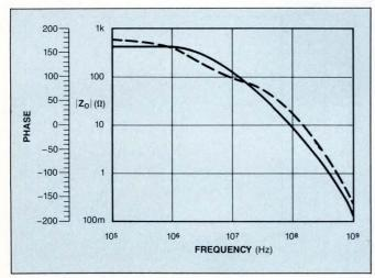
Fig 19—The compound pnp device has an excess phase of 160°. Its equivalent delay of 1.2 nsec is undesirable in feedback circuits.
