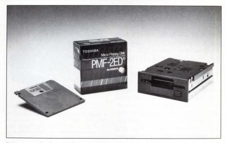
Using perpendicular-recording technology and a 34,868-bpi recording density, Toshiba produces the PD-210 2.95M-byte floppy-disk drive that maintains read/write compatibility with 720k-byte drives.
