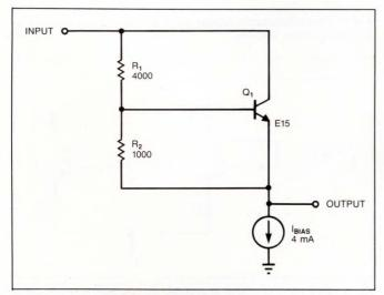
Fig 3—This  $V_{BE}$  multiplier is useful for noninteger multiples of  $V_{BE}$  or when available devices are scarce.
