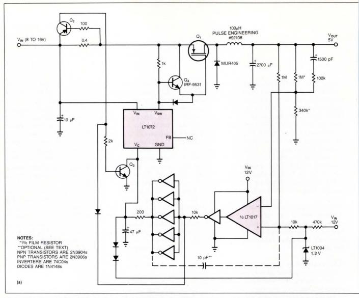
Fig 6—Using the special loop technique to introduce conditional instability works just as well in step-down converters (a). In transformer-coupled converters (b), you can use the loop technique to develop multiple outputs.
