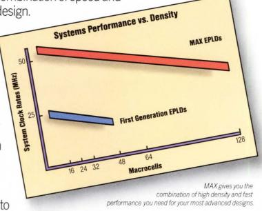
Which makes MAX the fastest, high density CMOS EPLD in the world. For example, with our EPM5032, you can design a bus controller that runs at 32MHz while utilizing 32 registers and up to 32 product terms feeding a single register.
