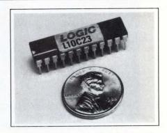
chip, and a compare-flag output pin will indicate if the 7-bit score exceeds the threshold value. You can cascade any number of L10C23s to search data streams for longer patterns such as 128 and 192 bits. The typical power consumption is 5V at 25 mA. The L10C23 is available in three speed ranges and comes in either a 24-pin ceramic leadless-chip carrier or a plastic DIP. \$25 to \$34.60 (1000).
