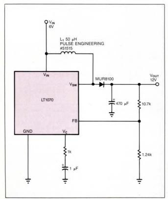
Fig 2—In this typical flyback-type converter, the LT1070's internal 40-kHz clock produces a flyback event every 25  $\mu$ sec. Each time the LT1070's  $V_{SW}$  pin internally switches to ground, it produces an inductive flyback voltage that converts the 6V battery input to a 12V output.
