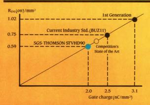
The Very High Density SGS-THOMSON STVHD90 (Blue dot) has a lower " $R_{\rm DS}$  On" resistance and gate charge than industry standard (Black dot).
