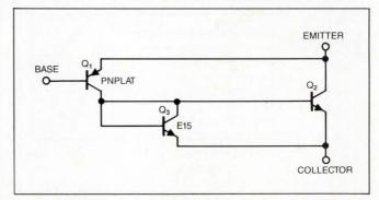
Fig 20—The presence of diode  $Q_3$  improves the operation of this compound pnp device. The  $f_{\tau}$  of this compound pnp is about 100 MHz, and its phase shift is a tolerable 35°.
