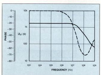
Fig 15—Plotted here is the output impedance versus the frequency for the circuit in Fig 14. The magnitude of the circuit's impedance continues through high frequencies.
