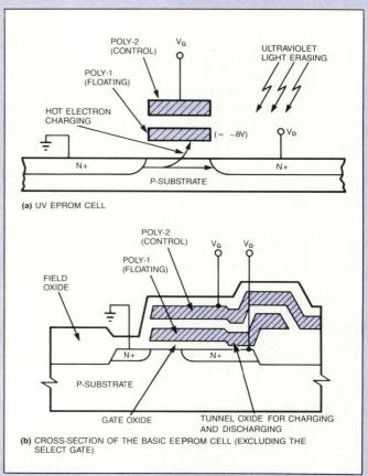
Fig A—As you can see, the differences between the conventional EEPROM cell and the UV EPROM cell are marked.
