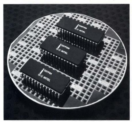
Flash EEPROMs can directly replace UV EPROMs. Intel's 27F64 and 27F256 are directsocket replacements for their 64k- and 256k-bit JEDEC-standard EPROMs.
