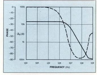
Fig 17—This plot shows the output impedance versus the frequency for the circuit in Fig 16.
