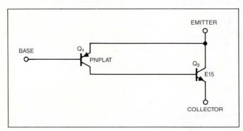
Fig 18—This compound pnp device combines an npn transistor and a lateral pnp transistor to form a high-beta pnp equivalent.
