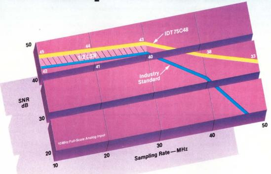
The IDT75C48 and 75C58 8-bit Flash A/D Converters, manufactured using IDT's CEMOS™ process, are pin and function compatible with the industry standard yet provide higher speeds, lower operating temperatures, and greater reliability.
