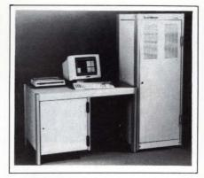
tion to functional verification, the system measures dc parameters. To test the dynamic (ac) properties of an IC, the system uses a "scan-ring" technique—it interconnects the scan circuits' inputs and outputs to form a free-running oscillator whose oscillation frequency is a measure of the device's speed. The system is based on an IBM PC/AT-compatible computer. It is modular in increments of 128 pins and can accommodate 1792 pins. Each module can contain four scan generators. The
