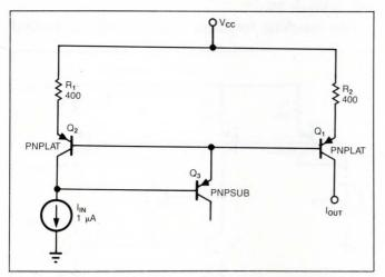
Fig 9—Because of the low beta of the lateral pnp devices, this simple pnp current mirror has an output-current error of about 4%.
