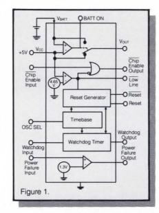
uncommitted 1.3V threshold comparator can serve as a power-failure warning indicator or monitor for the backup battery.
