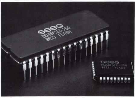
**The flash EEPROM** offers high bit densities and a chip-erase mechanism. Seeq's 48F512 is a 512k-bit device available in 32-pin ceramic and plastic DIPs as well as surface-mount packages.
