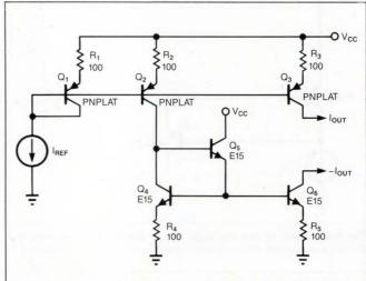
Fig 13—This circuit uses a matched pnp source as the reference for an npn current mirror. The total mismatch between the pnp source and the npn sink is about 2%.
