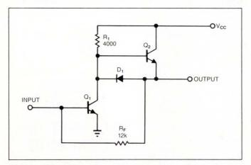
Fig 21—Although complementary npn-pnp transistors are often used for class B output drivers, this basic circuit uses only high-performance npn devices.
