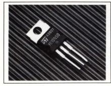
vice at frequencies as high as 10 kHz. Other features of the device include 100W maximum power dissipation, the ability to operate at a junction temperature as high as 150°C, and typical rise and fall times of 0.7 and 1.1 µsec, respectively. The STHI10N50 is available in a TO-220 or a fully isolated ISO-WATT-220 package. \$2.16 (100).
