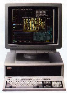
VAXstation 3000 VHDL Simulation 50,000 gates/4,000 vectors 15 min 31 sec
