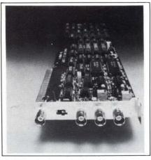
long as 32k bytes with an option that extends it to 64k bytes. Jumper straps allow the card to sample one channel at 40 MHz with 32k bytes of memory (or an optional 128k bytes), select X1 or X10 gain, and perform master/slave triggering for parallel channels. \$1395.
