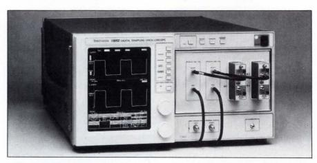
A touch-sensitive screen and rotary controls, whose functions depend on the menu from which you access them, give the 11800 Series scopes an uncluttered panel despite a wealth of firmware-resident features.
