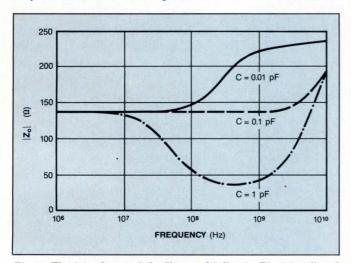
Fig 5—The impedance of the  $V_{BE}$  multiplier in Fig 3 is affected by the circuit's total collector-base capacitance.
