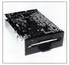
A magnetic servo signal buried beneath the magnetic data continuously keeps the 21.4M-byte Brier Technology BT 3020 drive on track and allows the drive to offer a 35-msec average-access time.
