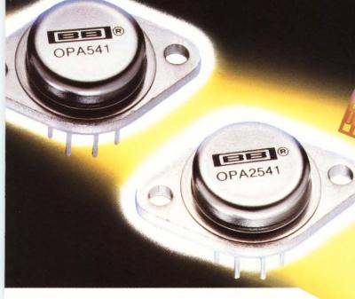
Our new OPA541 op amps deliver more power for your money, up to 5A continuous, 10A peak, from ±40V supplies. And OPA2541, the dual, saves valuable board space—especially important in multiple power amp applications. Use them as drivers for servo motors, ATE pins, voice coils, and power actuators.
