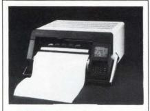
200 msec. It features trace annotation, trace overlap, retrace, and external synchronization facilities. The Model 520 is portable and operates from 110 or 220V ac line supplies or from a 10 to 32V dc supply. Options include an alarm module that detects and flags out-of-limit input signals. From £3500.
