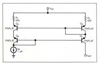
Fig 12-This Wilson current mirror has a high output impedance and slightly improved accuracy at low beta.
