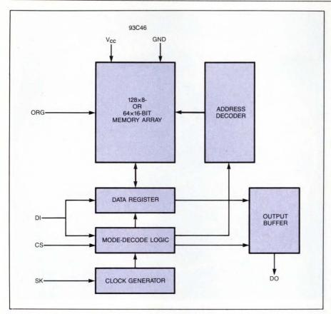
Fig 1—The 93C46 is representative of the industry-standard serial EEPROM. This type of device comes in an 8-pin package, yet differs in bit densities.
