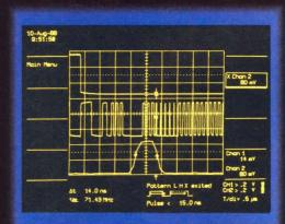
Logic conditions can be individually set for each of the 9450's inputs. PATTERN trigger mode is used to trigger only when the logic condition CH1 Low (top trace) and CH2 High (middle) is exited. The pattern must also be present for less than 15 nsec (lower trace). The trigger position is shown by the arrow at the bottom of the graticule.
