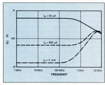
Fig 2—The impedance of the diode-connected E15 transistor varies with both frequency and current.
