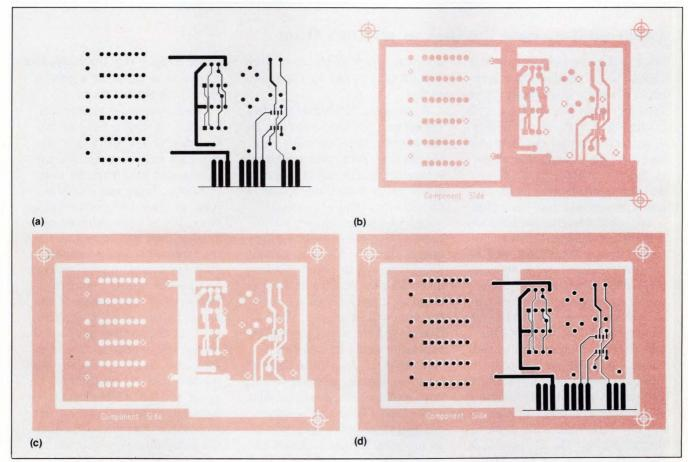
Fig 2—Being able to incorporate traces on a ground plane is important for many analog applications. First, you need to route the traces on the trace layer (a). Then copy this pattern and widen the traces and pads (b) and invert the image (c). Finally, combine the two patterns to make the composite image (d).
