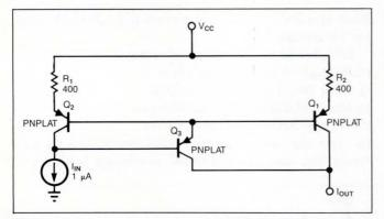
Fig 11—You can improve the accuracy of pnp current mirrors by adding transistor  $Q_3$ , which adds its collector current to the mirror's output.
