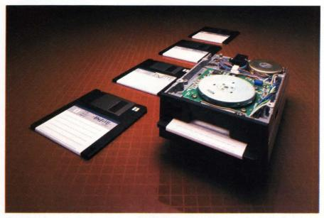
Servo tracks optically inscribed on standard floppy media allow the Insite Peripherals Floptical drive to store 20.8M bytes at a track density of 1250 tpi.
