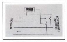
signals and performs the loopback in accordance with Bell PUB 43004. The XR-T2713 features a low operating current of 3.5 mA at 12V, pinselectable detection bands accurate to  $\pm$ 15 Hz, a detection level to -34 dB, and complementary TTL-compatible outputs. The device comes in a 16-pin DIP. \$5.02 (1000).
