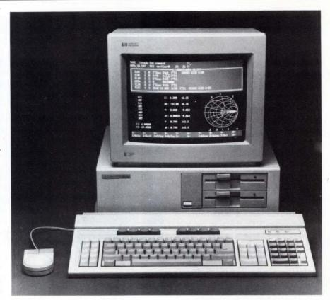
This microwave/RF simulator from EEsof Inc runs on IBM PCs and compatibles and handles striplines as well as networks.
