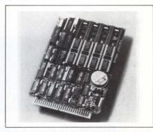
backed RAM. For non-STD DOS applications, you can use the board as a standard 1M-byte memory board. The board is compatible with the company's family of STD Bus CPU boards based on the 8088, V20, and V50 μPs. It is also compatible with boards that meet the STD-8088 specification. It contains eight 32-pin JEDEC sockets that accept either 28- or 32-pin EPROMs, EEPROMs, and static RAMs. \$395.
