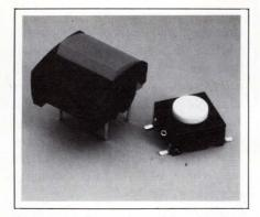
face mounting using pick-and-place equipment. They have a 10.1-mm-square footprint and a height of 6.4 mm. You can fit them with a range of standard or customized colored keycaps. The keycaps can incorporate a medium intensity LED indicator or high intensity illumination. The keyswitches have an operating force of 150 grams and provide 1 mm of switch travel with tactile feedback. \$0.65.
