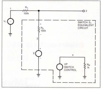
Fig 2—This Spice2 model is the equivalent circuit for the simple switch in Fig 1.
