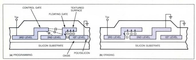
Fig 2—The textured-surface EEPROM cell uses three polysilicon gates. These Xicor cells make use of a thick tunneling oxide to charge and discharge the floating gate.
