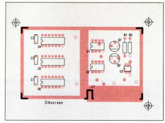
Fig 3—Split planes can be useful for accommodating both ground and power signals when you need to mix analog and digital grounds or when you need to isolate large areas.
