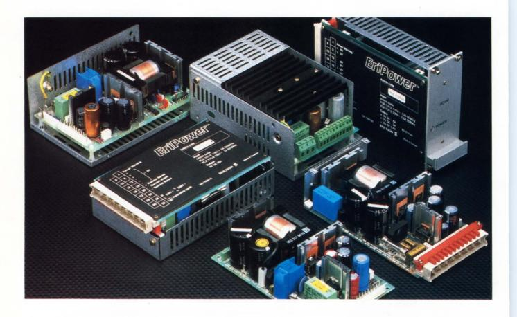
They're all reliable, with an MTBF of over 300,000 hours. They're all very compact and between 78% and 85% efficient. And, they all meet internationally recognized standards including VDE, IEC,
