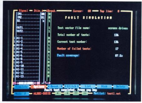
**Digital simulators** (such as this one from Aldec) may include built-in or optional fault simulators that indicate which pins of an IC fail the tests applied.
