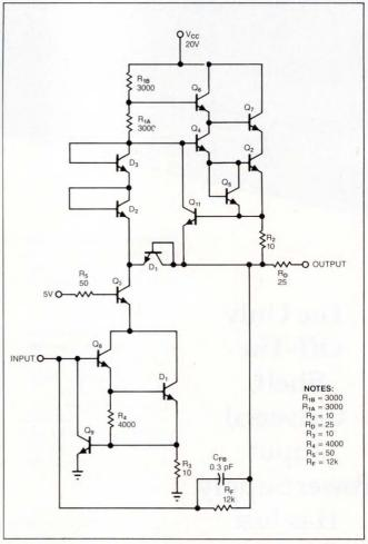
Fig 22—This practical implementation of a class B driver uses several additional devices to achieve high performance.
