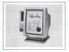
dots/in., and a letter-size resolution displays  $640 \times 870$  pixels, using 80 dots/in. The letter-size model displays a single-page document on the screen. Other features include a noninterlaced screen refresh rate as fast as 97 Hz, a full tilt-and-swivel base, and contrast and brightness control switches. The software lets the user switch between the two
