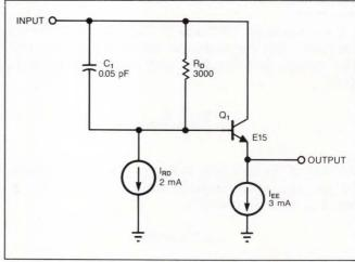
Fig 7—This level-shifter circuit has low dynamic impedance and good temperature stability.
