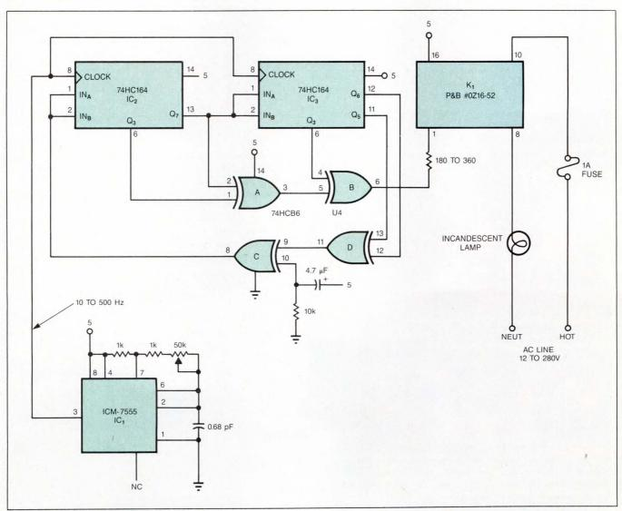
Fig 1—This pseudorandom sequencer can produce a realistic flickering in incandescent lamps that is similar to the flickering of a flame in the breeze.
