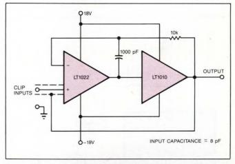
Fig 1—You can solve a lot of loading problems by using this simple probe, which employs an LT1022 high-speed FET op amp to drive an LT1010 buffer. The LT1010's output serves as a cable and probe drive source, and it also biases the circuit's input shield.
