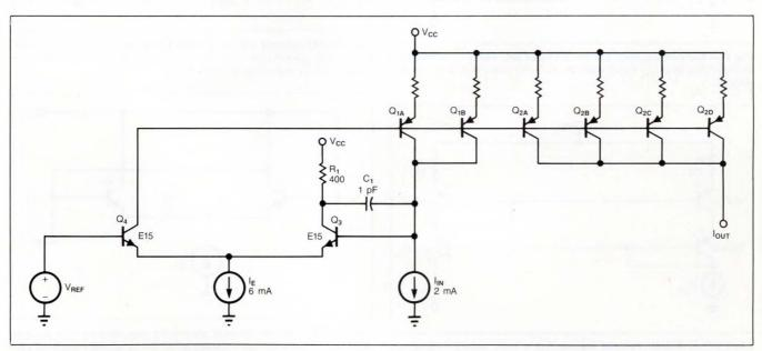
Fig 10—This pnp current source uses an npn control amplifier. This circuit is useful for controlling relatively high-current pnp sources.
