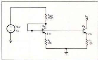
Fig 8—This current source is suitable for driving the level shifter in Fig 7. You can use multiple current sources to drive additional level shifters.
