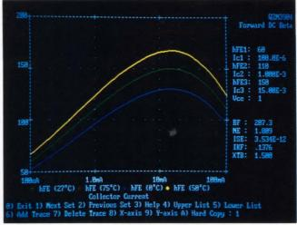
Characterizing a Transistor with Parts
