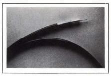
layer foil bonded to the dielectric core followed by an aluminum-braid shield and then an overall copolymer mylar foil. The outer foil has a shorting fold, which provides metal-to-metal contact for maximum shield effectiveness. Both cables are available in 1000-ft put-ups. \$220.65 and \$377.25 for the 1223A and 1224A, respectively.
