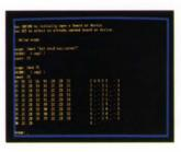
Applications Monitor— A utility that performs automatic error detection and identification. For ease in debugging, a Session Summary of all the GPIB commands made during a session is generated.
