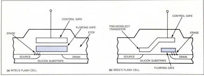
Fig 3—Although flash EEPROM cells differ in structure, they do have commonalities. The floating gate is charged using hot electrons and is discharged via Fowler-Nordheim tunneling.
