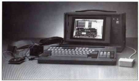
1.2M-byte 5½-in. floppy-disk drive, a 20M-byte hard-disk drive, and an 86-key keyboard. The 16-MHz 80286 version, from \$4270; the 20-MHz 80386, 4.5-MIPS version, \$7470.
