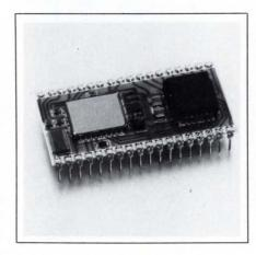
handsets, the PBL3726/19 telephone speech-circuit IC features soft clipping to reduce distortion at high speech levels. Automatic gain control reduces the gain of the transmit amplifier by as much as 5 dB when the ac signal on the telephone line increases to 2V peak.
