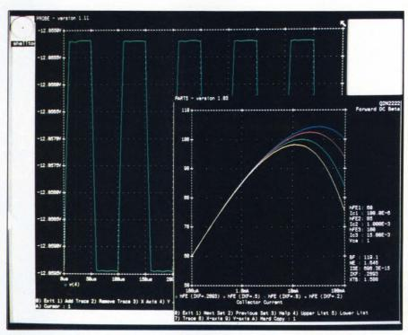
Interactive analog simulators, such as PSpice from Microsim Corp, let you see the results of changes in circuit parameters immediately.
