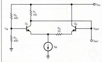
Fig 14—This all-npn current source for pnp devices uses positive feedback to increase the impedance of  $R_1$ . A disadvantage of this circuit is its small voltage compliance, which is approximately  $I_E R_2$ .
