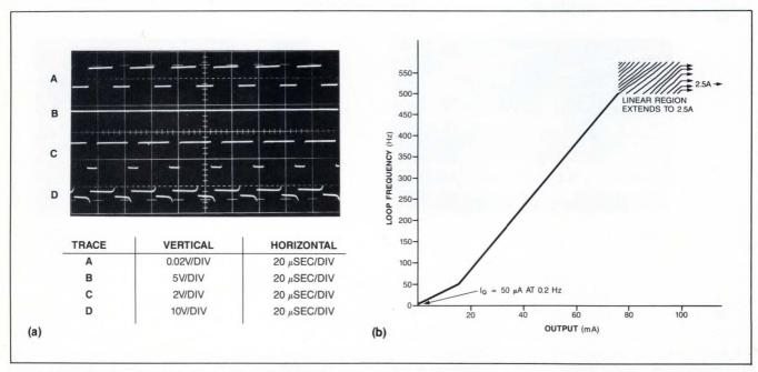
Fig 4—When you look at the waveforms for a 1A load, you see that the  $V_C$  pin is at dc and the repetition rate now equals the LT1070's 40-kHz clock frequency (a). As the loading increases (b), the loop oscillates at a higher frequency because of  $C_1$ 's decreased decay time.
