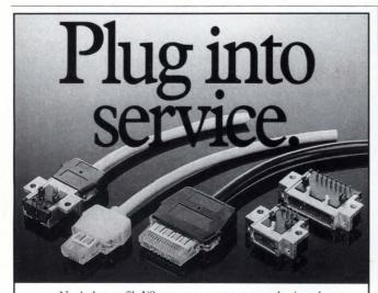
Need a low profile I/O connector system you can plug in and forget? Take a look at Compu-Shield. It's a fully modular system of demonstrated reliability, featuring a proven contact system. Contacts are on .050 in. centers, with 360° shielding against EMI/RFI for data busing. Selective gold plating in the contact area maximizes conductivity while keeping costs down. The spring contacts are totally enclosed and tension pre-loaded.
