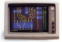
For starters, Master Designer's schematic capture and interactive layout lets you design using the latest through-hole and surface mount technologies.
