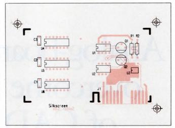
Fig 1—Most pc-board CAD packages allow the user to add copper and guard signals. Notice the shielded trace on the right side.
