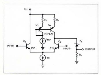
$\textbf{\it Fig 6--A zener-diode level shifter} \ is \ driven \ from \ a \ high \ impedance \\ source.$
