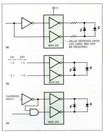
Fig 1—The simplest circuit, (a), lights one LED or the other. The circuit in  $\mathbf{b}$  allows you to light one, the other, or neither, while  $\mathbf{c}$  provides an override function.
