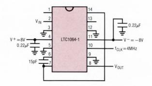
Figure 3. The LTC1064-1, Monolithic 8th Order Cauer Low Pass Filter Operating with a 4MHz Clock and Providing a 40kHz Cutoff Frequency
