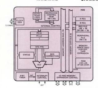
Supplier says it uses a "strip-chip" architecture to keep registers and control elements in isolated, self-contained modules in silicon, and then it uses single layer of metal to interconnect chip. This is, of course, similar to the cell-library, semicustom approach and useful for the same reason. Changes can be made easily, which helps TI bring out new models or give large customers special variants.
