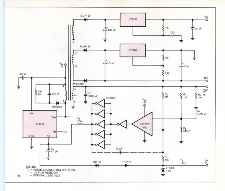
that of Fig 2a because of the lower output voltage. In other respects, the loop and its performance are identical to those of Fig 2a. Fig 6b shows how you can use this loop concept in a transformer-coupled converter. Note that the floating secondaries allow the circuit to generate a  $\pm 12V$  output.
