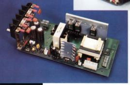
Top PC board showing power transformer and rectifiers.
