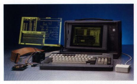
Bundling a logic analyzer on a PC bus card with a "luggable" PC, as Dolch does with its Cobra-PA480, creates a portable system with lots of expansion potential.
