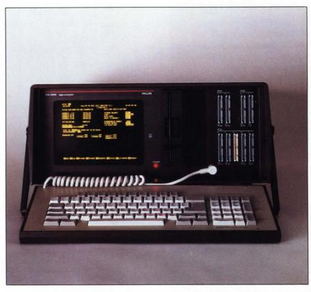
It's possible to design a PC around a logic analyzer, as Philips has done with the PM 3655—sold in the US by John Fluke Mfg Co.
