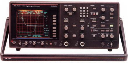
PM 3340 2 GHz repetitive signal digitizing oscilloscope with full range triggering, 1 mV/div input sensitivity and 1.6 V dynamic range for signal detail
