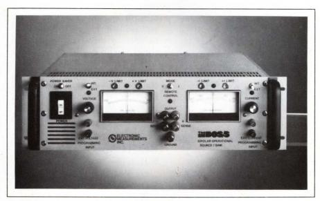
tions have 12-bit resolution. Voltage and current regulation is 0.005%. TC is 0.01%/°C in the voltage mode and 0.03%/°C in the current mode. RMS ripple equals 3 mV in the voltage mode and 0.05% in the current mode. Voltage and current output changes over 8 hours are 0.02 and 0.03%, respectively.
