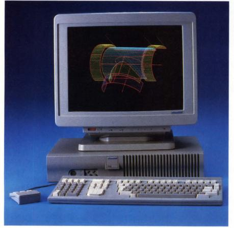
A redraw rate of 40,000 vectors/sec and the flexible connectivity scheme make the 4211 graphics terminal as functional as many workstations.
