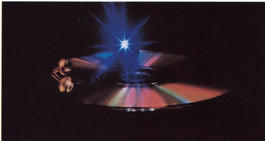
Aimed at the optical disk marketplace, the blue-light laser from Matsushita lases in the 390- to 420-nm wavelength range. Compared to the 780-nm lasers currently used with optical disks, the devices quadruple disk memory capacity.
