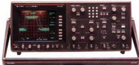
PM 3320A Single event digital storage oscilloscope with 250 MS/s sampling (catches 3 ns glitches), 200 MHz bandwidth and 10 bit vertical resolution
