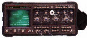
PM 3256 75 MHz, compact field oscilloscope
