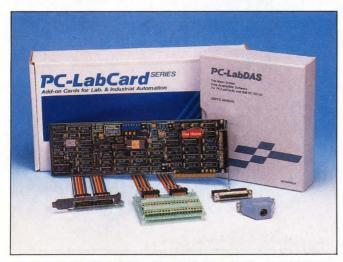
Low-cost, high-speed 12-bit analog I/O is available on the PCL-718 board manufactured by American Advantech. The 100-kHz card offers 16 single-ended or eight differential input channels and two analog-output channels.
