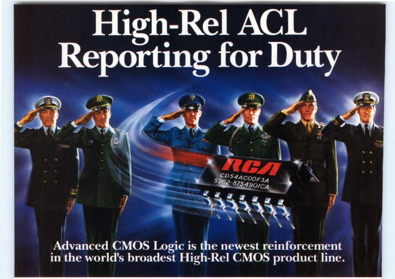
If you're designing tactical military systems, it's more logical than ever to come to GE Solid State for all your High-Rel logic needs. Because we've just introduced well over 50 ACL logic devices that give you the speed of FAST† plus all the benefits of CMOS. These devices, fully compliant to Mil-Std-883 Rev C, are available in both AC and ACT (TTL-compatible) versions.
