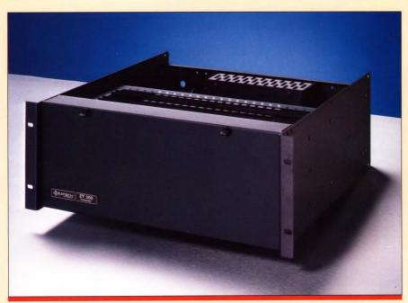
The ZT 300 is an integrated STD Bus computer featuring Ziatech's new version of STD DOS. The new STD DOS II allows Ziatech computers to run PC software programs like 86-Ladder and MICRO-VIEW.
