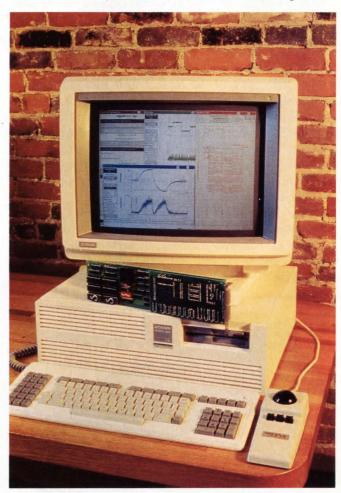
High-end workstations offer advantages in analog-I/O processing. Intended for Apollo's DN3000 and DN4000 workstations, the hardware and software products produced by SignificAT take advantage of the computers' extensive windowing, multitasking, and networking capabilities.
