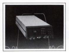
lows 5-year storage of eight complete 6-parameter setups on each of the two channels. You specify the unit to contain two filters with any combination of the following characteristics: 8-pole Butterworth lowpass or highpass, 8-pole/6-zero elliptic lowpass or highpass, 8-pole Bessel lowpass, or 8-pole/6-zero constant-delay lowpass. The last-
