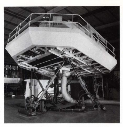
Employing about forty 80286-based CPU cards, Singer Link-Miles' flight simulator for the A300 Airbus contains one of the largest Multibus II computer systems yet constructed.
