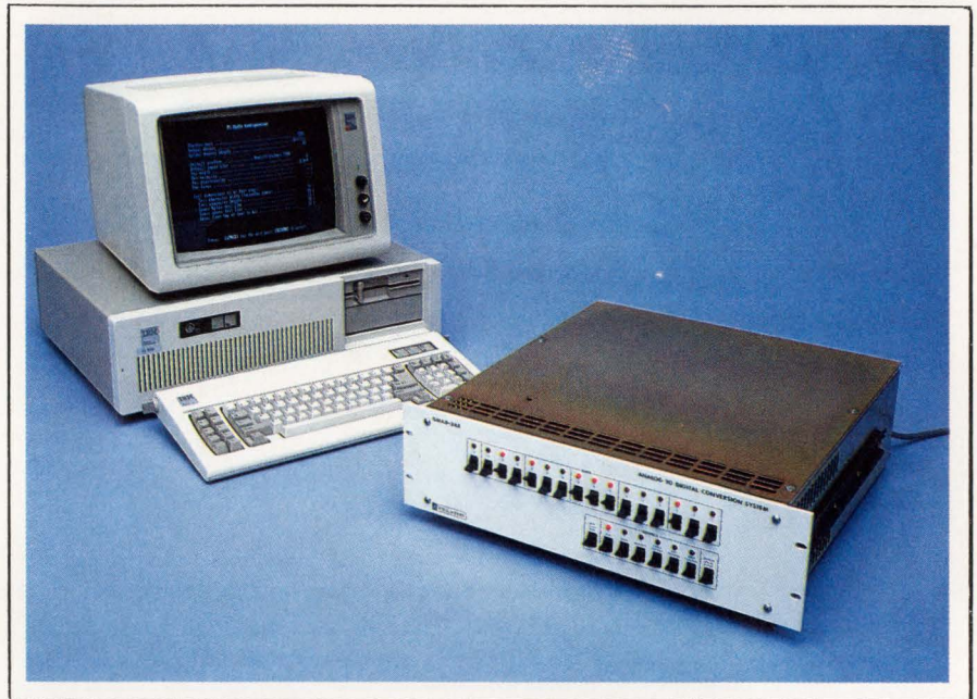
Providing a \mu P-controlled IEEE-488 interface to your PC and instruments, this A/D-conversion system from Preston Scientific helps you integrate GPIB control with data-acquisition tasks.
