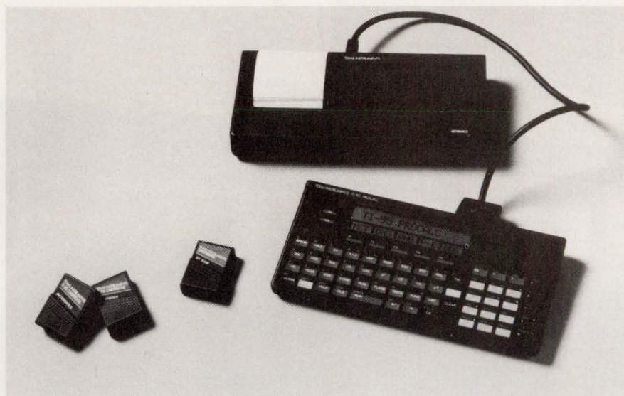
The $200 TI-95 from Texas Instruments requires only a simple connecting cable to drive its companion printer ($115). The calculator also accepts preprogrammed ROM cartridges containing applications programs or constant-memory cartridges for storing user programs and data.
