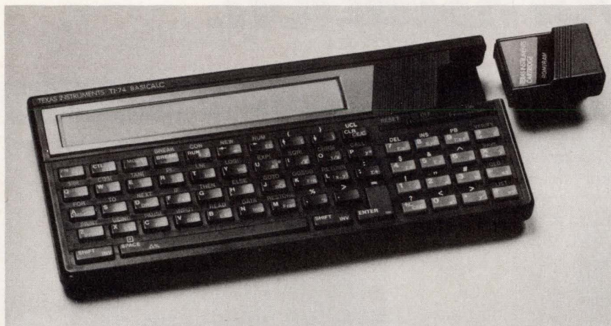
The press of a button switches the Texas Instruments $135 TI-74 from a handheld Basic computer with scientific functions to a scientific calculator.
