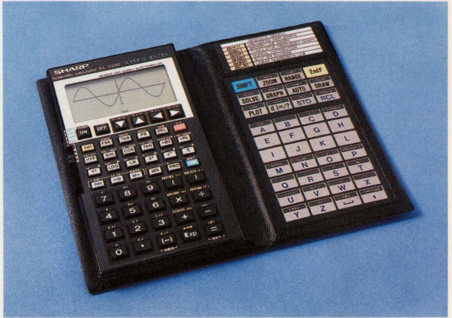
A powerful Zoom key for manipulating graphs is one feature of the $109.95 Sharp EL-5200. Other graphical calculators require you to call up and alter the Range menu for scale changes.
