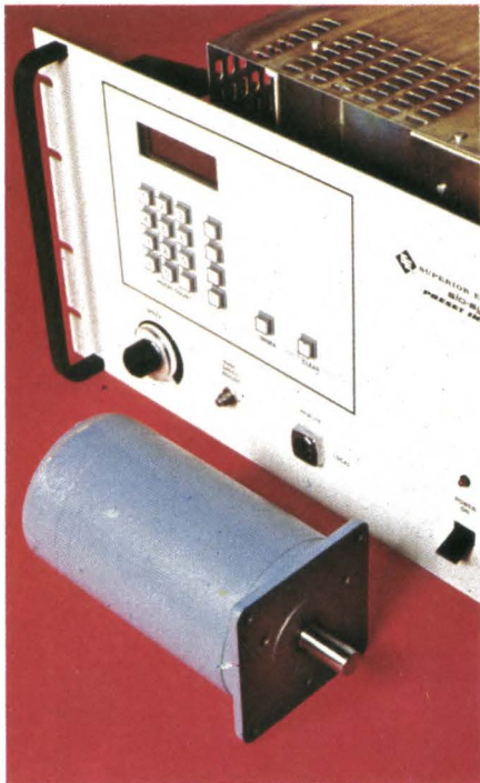
A preset indexer from Superior Electric, Model IK600 drives a 0.8-hp stepper in response to an operator keyboard command. This \mu P-based controller features adjustable minimum/maximum frequencies and acceleration/deceleration rates for optimizing motor performance.
