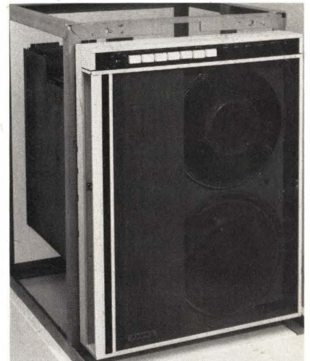
A 7- or 9-track tension-arm unit, Ampex's TM-E Mod 5 records in NRZI or PE modes and reads bidirectionally.
