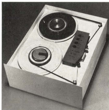
Employing \mu P control, Kennedy's Model 6809 Data Streamer transport eliminates conventional tape-tensioning elements.
