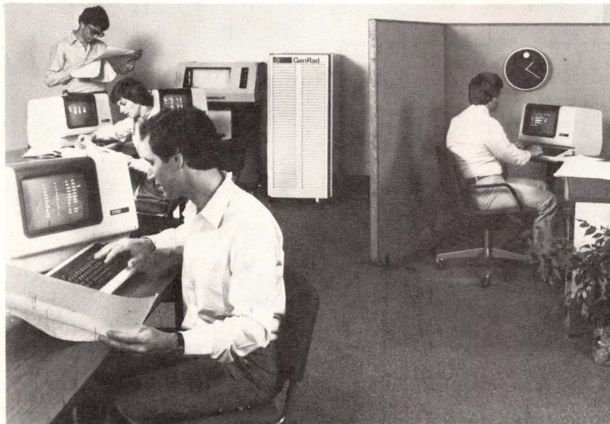
Four programmers can share this GenRad 2290 in-circuit test-generation station.
