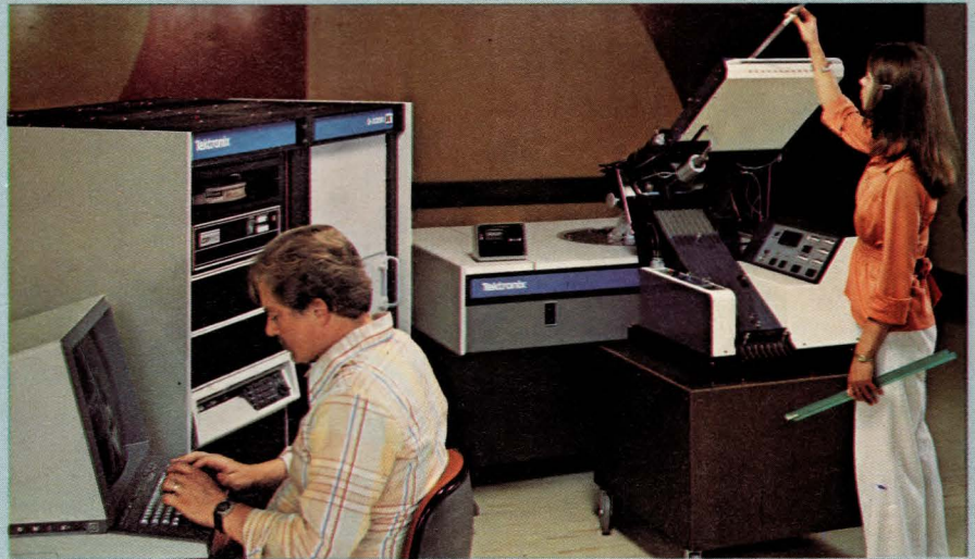
Computer-aided program-generation software provides the skeleton for testing high volumes of relatively simple SSI and MSI devices on Tektronix ATE systems, such as Model S-3250.
