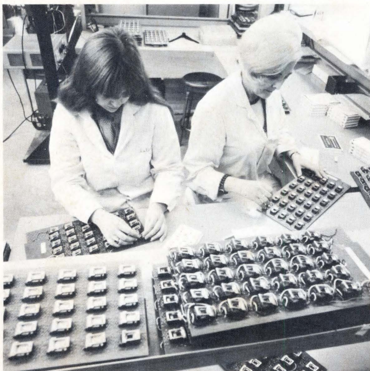
To make room for instruments? Some of the 40,000 test sockets in Associated Testing Laboratories screening facility.
