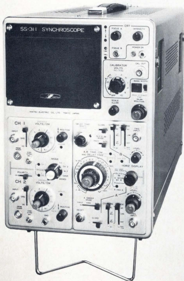
The Iwatsu SS-311, marketed here by E-H Research Labs, now enjoys the speed lead, with a bandwidth of 300 MHz and top-frequency sensitivity of 10 mV/cm.
