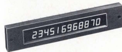
Burroughs Panaplex panel display uses 9 segments per character. A 12-character display is only 6.2 inches long, 1.62 inches high and 0.4 inches deep.
