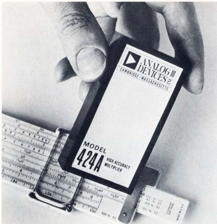
Analog Devices' new analog multiplier has an accuracy of 0.1%, and a bandwidth of 100 kHz, yet it is less expensive and more compact than other computer-grade units.
