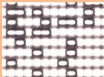
Fig. 2. Photomicrograph of the EA 3501, a 512 by 5 MOS read-only memory, which is coded as an ASCII to 5 x 7 dot matrix character generator. A portion of the memory matrix is enlarged to show the memory cells in more detail. The
