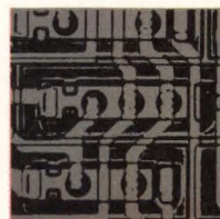
ENCODERS 9318 — Priority 8-Input Encoder
