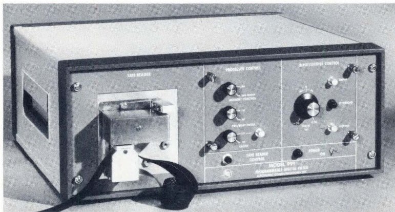
ECI's digital filter, programmable with paper tape.
