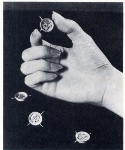
New power hybrid IC developed by RCA.
