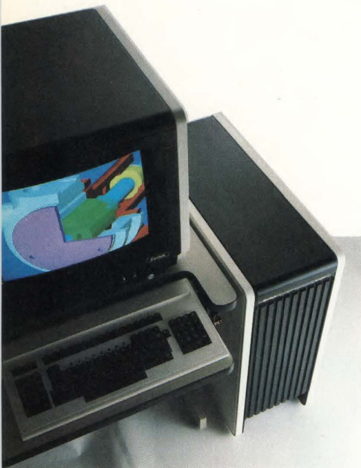
Ramtek's 9645 may be a 16-bit display processor, or a 32-16 bit system with up to 5 68000 based cards for graphics operations.
