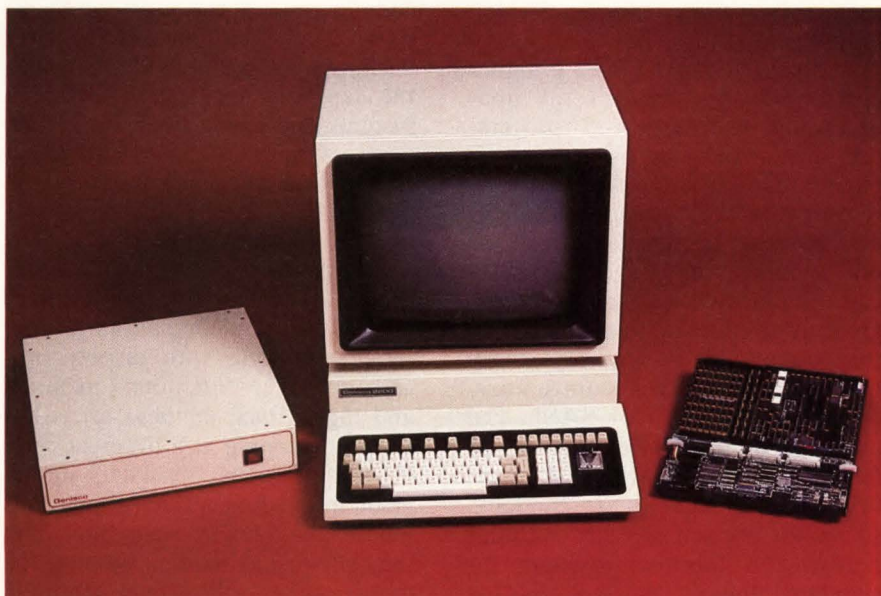
The G-2000 Product 1 line from left to right configured as an OEM product, a stand-alone graphics system, and a system component for display processing, demonstrating the flexibility offered to manufacturers with today's display processors.
