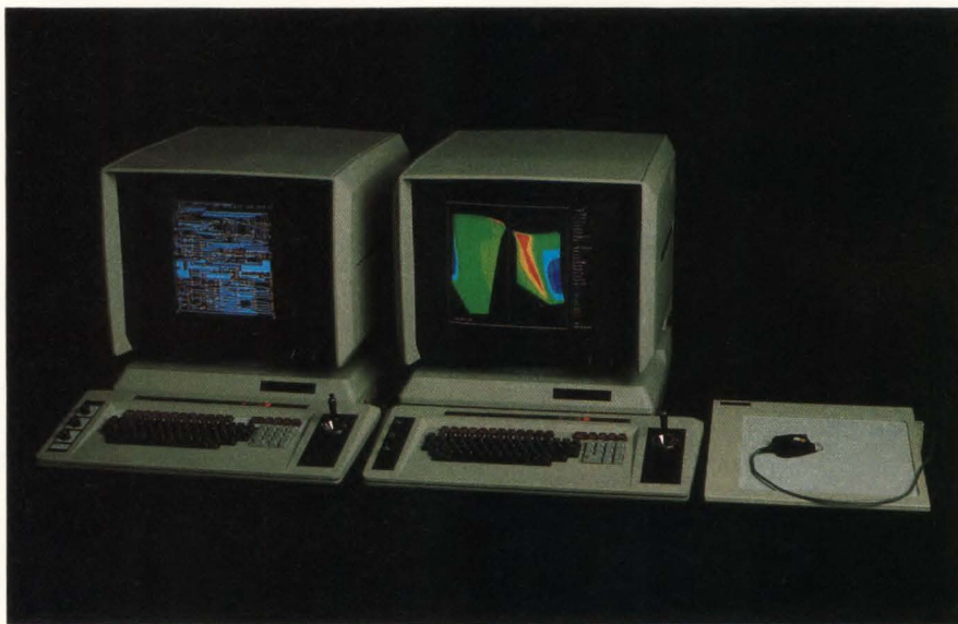
The Megatek 7200 Graphics Engine's PC layout and computer aided engineering displays. The system has both a 32 bit system bus and a 16 bit peripherals bus.
