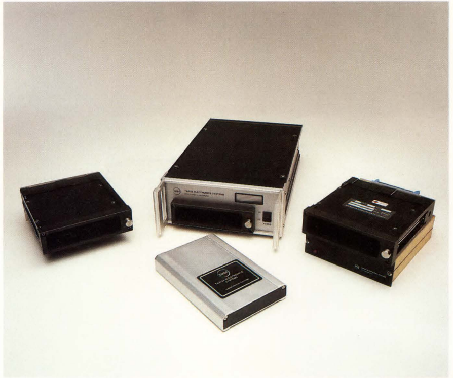
Figure 2: The data recorder, floppy emulator, and cartridge holder all use the same removable cartridge.
