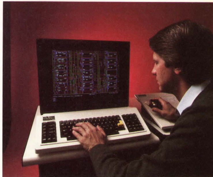
Figure 9: Daisy Systems' Gatemaster work station dedicated to gate array design. Station is used for schematic capture, simulation, layout and verification.
