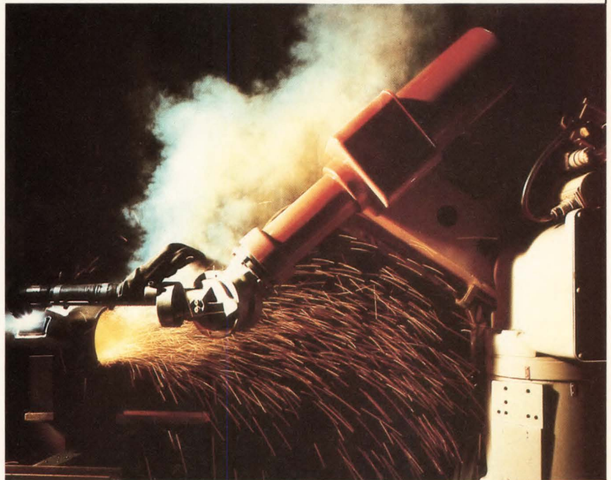
Cincinnati Milicron's electric-driven T 3 -726 Robot performs a plasma arc cutting operation on a steel pipe.
