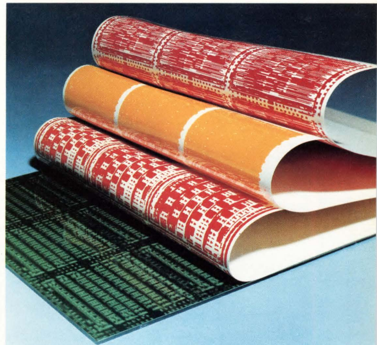
Figure 2: Motorola metalization mask patterns. Company's MOSAIC process is used to fabricate low power Schottky arrays, including MCA2800 ALS as well as ECL arrays. Three masks are required: one for each metal level and one for via holes.
