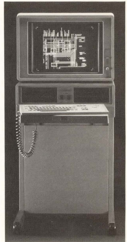
Figure 1: The Model 4115 computer display terminal features a high performance color raster scan display which displays 1280 \times 1024 pixels at a 60 Hz non-interlaced refresh rate.
