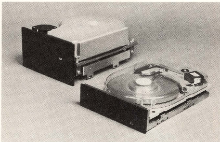
Figure 1: Decreased height in today's half-height Winchester drives (such as the Shugart SA706, above right), as well as in flexible disk drives, resulted primarily from a streamlined DC spindle motor design.
