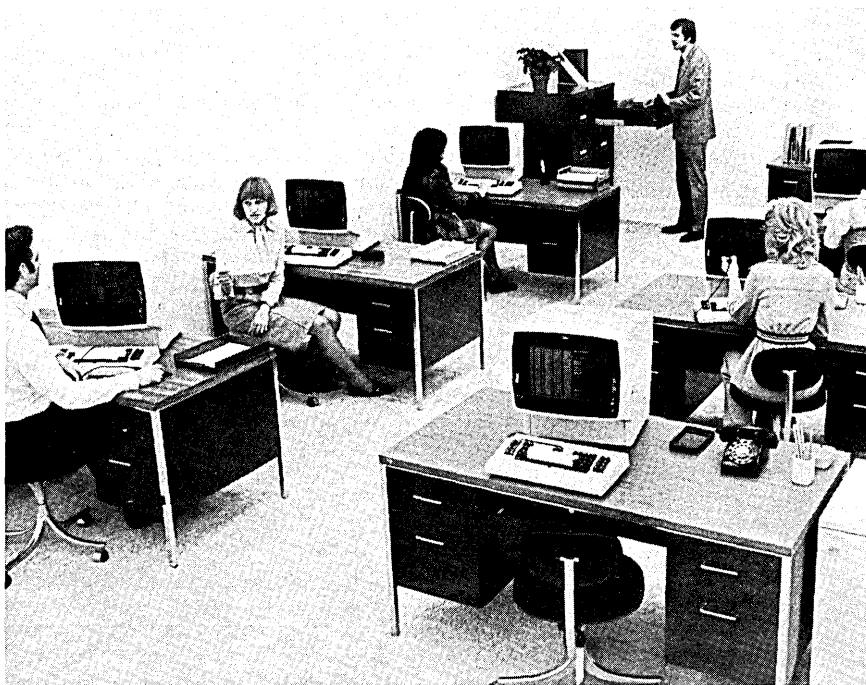
Announced last May, the IBM 3278 display station, shown here in design models, can be grouped in clusters of up to 32 units in a BSC or SDLC network. Four screen capacities are offered with the largest allowing a display of up to 3,440 characters.
