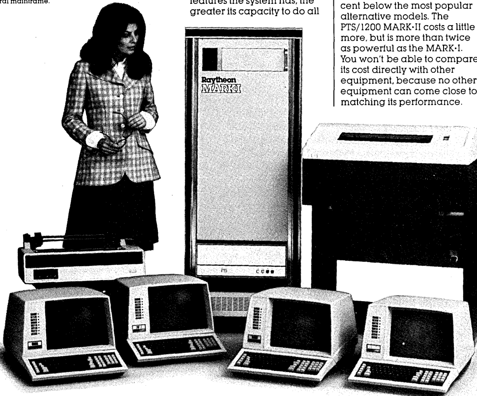
A typical four-station MARK-I system with a 64K-byte controller, 10 MB disk, and one 165cps printer leases for $850 per month, including all software and maintenance.
