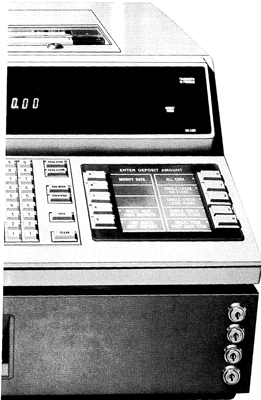
Shown above, the NCR 270 financial teller terminal with full keyboard. Ten-key and alpha-numeric keyboards are also available.
