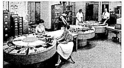
Oil Refinery Rotaries speed IBM inventory system with fast access to 30,000 punch cards.
