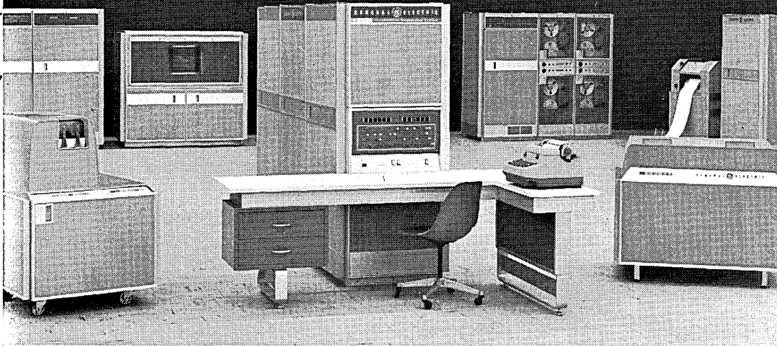
GE-225: Medium-sized, versatile system; 18 microsecond word time.
