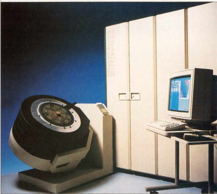
Teradyne's J971 series of VLSI testers uses a combination of proprietary E/MOS technology and plug-in hardware upgrades called performance cells to cut costs by about half over the previous generation of test equipment. An interactive graphics software package streamlines the process of developing test programs by separating test parameters and test data definitions from the creation of program code.
