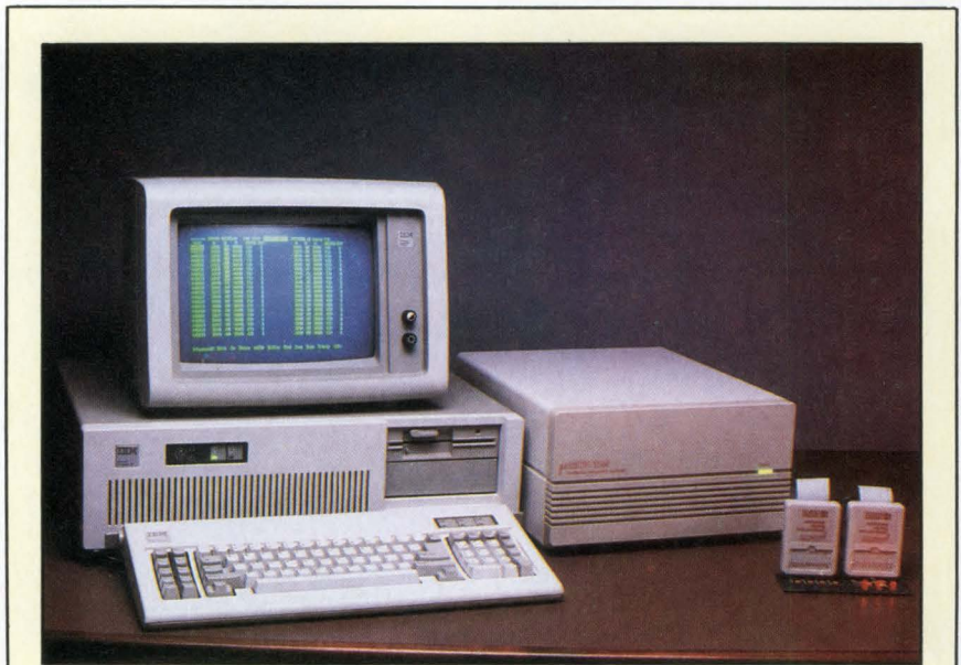
Northwest Instruments' MicroAnalyst workstation consists of an IBM PC AT, Northwest's Series 2000 logic analyzer, and Lotus Symphony software. The system is competitively priced with many standalone logic analyzers.
