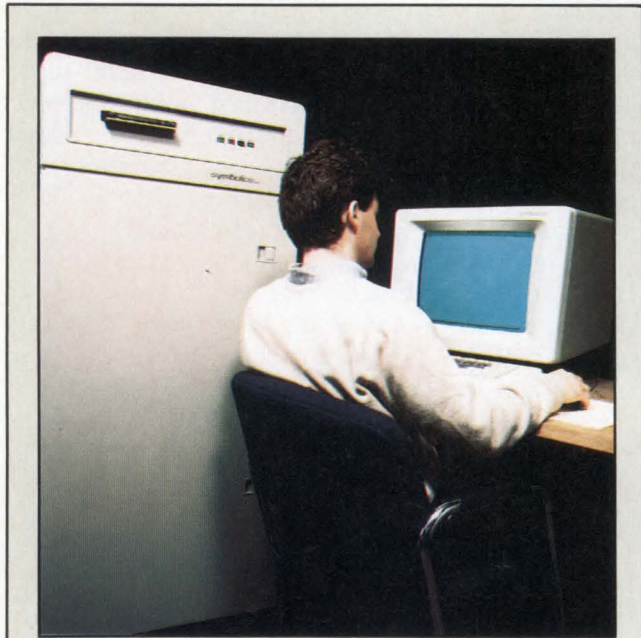
The high end Symbolics 3670 symbolic processing workstation has all the hardware needed to support a Zetalisp environment. Flavors, an object oriented Lisp extension, and a variety of integrated Lisp based software tools such as editors, windows, compilers, and debuggers, are also provided.
