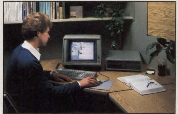
Tektronix, Inc is making its mark in the world of symbolic processing workstations with its 4404. Designed around the Motorola 68010 and the graphics oriented Xerox Smalltalk-80 programming environment, the workstation is geared to help hardware designers.
