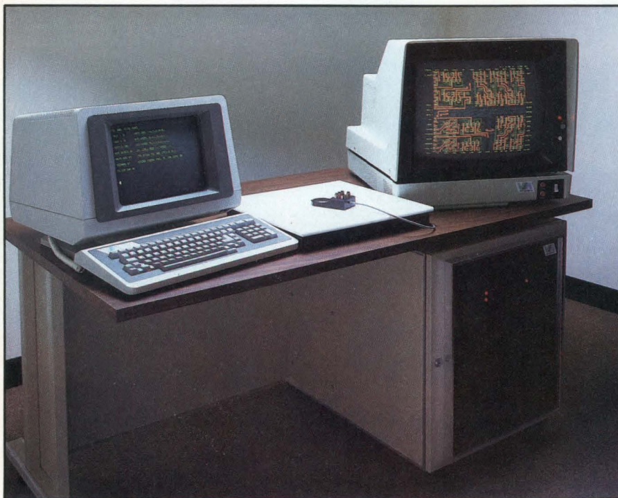
A section of a typical custom IC circuit appears on the VIA Systems, Inc (N Billerica, Mass) Model 110 color graphics screen. The Model 110 is a single-user, color, interactive graphics system for IC design. It features a high resolution 19" color graphics screen with 16 colors, 3 computers, and over 700,000 bytes of memory.
