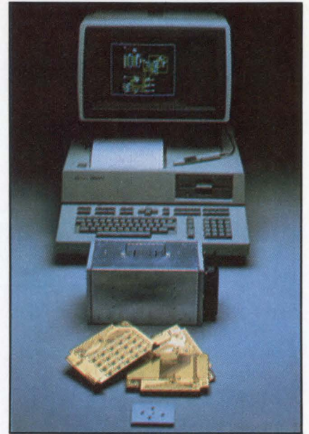
Five-chip set in foreground mounts on boards (above chip set) as nucleus of 32-bit HP 9000 computer. Module in center is rackmounted version; background unit is standalone workstation.
