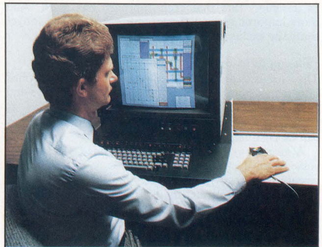
CAD systems such as VLSI Technology's integrated design system are the driving force behind growth in custom circuit design. As shown on the screen, IC designers can create stick diagrams using the STICKS graphics editor. Diffusion (green), polysilicon (red), and metal (blue) layers are easily differentiated in the color presentation.
