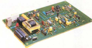
Remote Monitoring Equipment Modem
