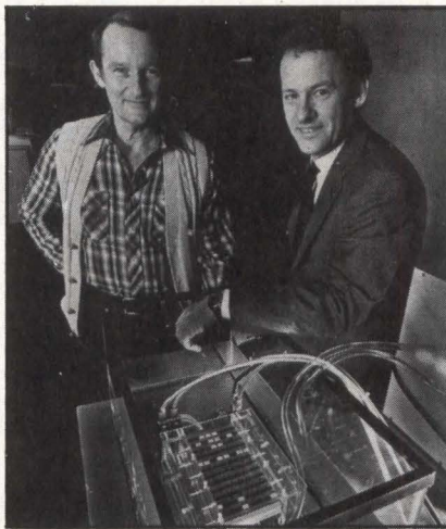
3-Dimensional module provides circuit density necessary to achieve CRAY-2's supercomputing speeds. Seymour Cray and John Rollwagen are shown with tank of inert liquid containing prototype module. Liquid immersion technology efficiently cools circuits within the module.
