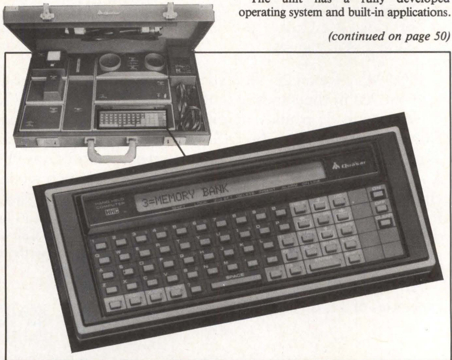
Handheld computer from Quasar puts processor, memory, printer, modem, and battery pack in an attache case. Programmable in SNAP and BASIC, unit connects to mainframes over telephone lines and to TV for local display.
