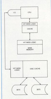
Memorex's 3770 disc cache increases performance of I/O bound mainframes by providing rapid CPU access to disc stored data. Using CCDs for dense mass storage, cache's microprocessor contains algorithm which maintains control of I/O requests
