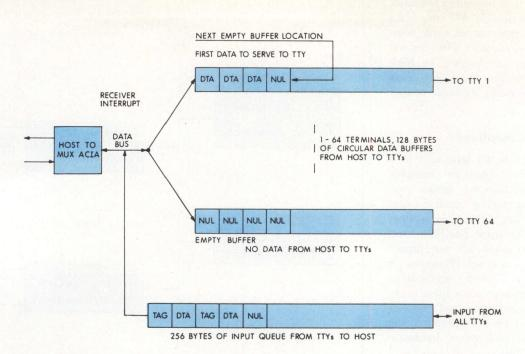
Fig 4 Address processing. Addressing information is transmitted to host with data each time for demultiplexing purposes. Demultiplexing rule can be dynamically updated for additional or fewer terminals upon reset. Receiver interrupt obtains data from host and places data in appropriate TTY output buffer. Same interrupt routine also services TTY input buffer to host. Therefore, fast I/O rate is produced between host and multiplexer
