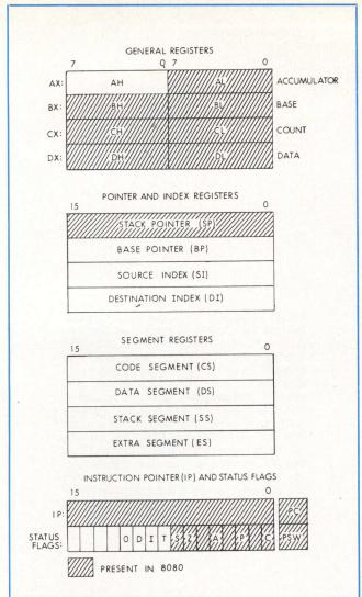
Fig 6 8086 register organization. Register structure of 8086 has seven more registers and four more flags than 8080. Major difference is that extra registers can process 16-bit data. However, general registers remain 8-bit byte addressable
