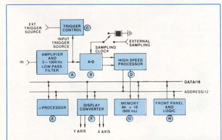
Key hardware elements in Rockland System's 7530A spectrum analyzer are (A) low noise, high sensitivity amplifier and 120-dB/octave low pass filter; (B) 12-bit linear A-D converter; (C) trigger control; (D) CPU that first bandpass filters input signal and then performs FFT spectrum analysis on it; (E) CPU that interprets front panel controls; (F) display converter; and (G) 8k x 16-bit memory formed from 16k-bit chips
