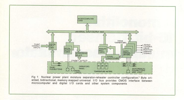
Physically the bus consists of printed circuit back-planes and flat cables to provide an uninterrupted, hardwired conductor for each signal or power line. Electrically it is a byte oriented CMOs interface with 1/0 cycles of 10 to 15  $\mu$ s. Printed circuit cards can be mixed anywhere on the bus.
