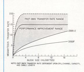
Using 1.2M-byte/s transfer rate, 4k block size, and single-byte wide transfer, Intel's FAST-3805 semiconductor disc is 3.5 times faster than IBM's 3350F disc system and twice as fast as 2305-2. Steep climb in 3805 curve is due to unit's 0.4-ms access time
