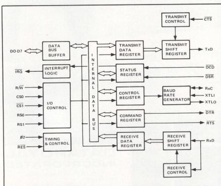
Asynchronous communications interface adapter device, Rockwell's R6551, provides 8-bit microprocessor based systems with UART interface for serial communication to terminals, data sets, and modems. Device is member of R6500 microprocessor family and is also compatible with 6800 based microcomputers
