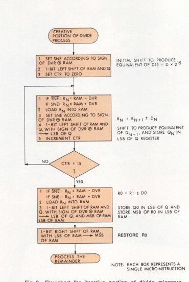
Fig 2 Flowchart for iterative portion of divide microprogram. Operations performed within each microinstruction are numbered to show execution sequence
