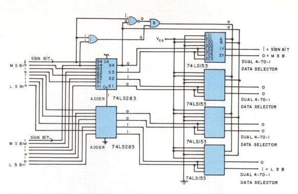
Fig 4 Overflow detector circuit. When addition of two positive numbers produces negative number, or two negative numbers produce positive number, overflow is detected. When detected, output sum is forced through 4-to-1 data selector scheme and is represented as either negative or positive maximum, depending on sign bit. For example, addition of 1 0101110 and 1 0110101 results in overflow; therefore data selectors switch to maximum negative 1 0000001
