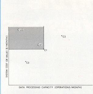
Fig 2 Matching system to user requirements. With each user and computer system represented by point, note that computer can profitably serve any user appearing above it and to its left on the graph. Computer C1, for example, has sufficient power to serve any user in shaded area, and costs less than value of all user applications in that area. Note that systems C2 and C3 cannot economically serve user U1, but can serve U2
