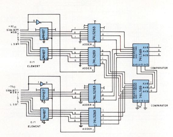
Fig 5 Magnitude comparison using standard IC comparators (7485). Conversion to signed magnitude number is needed before actual comparison. Conversion can use adder circuit configuration of either Fig 1 or 2. For wider word sizes (greater than 16 bits), comparison may require excessive hardware, and propagation delay is increased (unless high speed circuit of Fig 2 is used)
