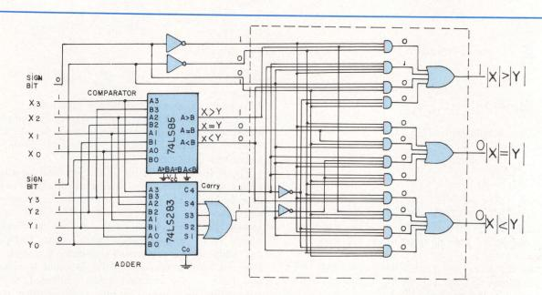
Fig 6 Improved magnitude comparison circuit. Magnitude comparison is performed by either comparison or addition. Propagation delay is therefore equal to delay in comparators or adders, whichever is larger. Logical manipulations are performed in last stage to give correct result. Logical gates could be integrated into custom IC for use in conjunction with existing comparators and adders to increase speed and reduce hardware
