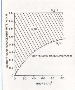
Fig 3 Replacement rate, without (upper curve) and with (lower single-error correction. curve) Rate is constant (with no error correction) because of assumption of a Poisson process governing chip failure rate and increases from zero to a constant value with single-error correction. Difference between two curves is decrease in replacement rate due to singleerror correction. Decrease becomes less as time progresses, tending to a constant value
