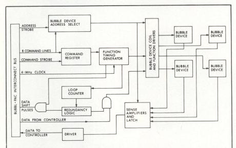
Bubbl-Tec's memory system consists of controller and Bubbl-Pac bubble memory module (diagrammed) that is replicated up to 16 times. System performs write, seek, and read operations; it is easily incorporated into any LSI-11 microcomputer requiring reliable, nonvolatile memory without moving mechanical parts
