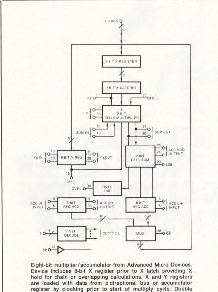
length 16-bit output is multiplexed onto 8-bit bus with either upper or lower half of result readable at any one time
