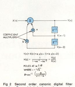
Fig 2 Second order canonic digital filter section. Boxes labeled z<sup>-1</sup> are storage registers that delay output sample words by one sample period
