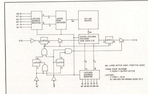
Fig 2 Individual RAM used in array is HM-6504, shown in this logic diagram. 16 of the 4k x 1 CMOS memories, in leadless carriers, are mounted on ceramic substrate. Design emphasizes advanced packaging techniques
