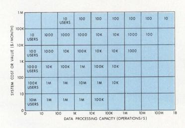
Fig 3 Potential users vs system value/capacity ranges. If each potential U.S. DP user is plotted as point on value/capacity graph, result is an estimate of number of points (and thus number of potential customers) in each value/capacity range. Numbers in squares are author's estimate, to nearest power of 10, of how many locations in U.S. could use DP capacity in range indicated by abscissas, and could afford to pay amount indicated by ordinates of square
