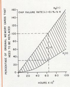
Fig 2 Percentage of original memory card population that needs to be replaced, without (upper curve) and with (lower curve) single-error correction. Difference between two curves represents percentage of card replacements saved due to single-error correction. Notice that by about 65,000 h, without error correction, each original card needs to be replaced once, whereas with single-error correction slightly over 30% of original cards need be replaced by this time
