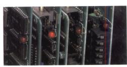
board. As each board is tested, a small LED (Light Emitting Diode) attached to the board's edge comes on. In a few seconds, if the board passes, its LED goes
