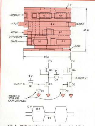
Fig 4 Shift register memory cell used in LSI implementation of digital filter. Bit is stored in parasitic capacitance C1 when clock  $\phi 2$  occurs, and is transferred to capacitance C2 on clock  $\phi 1$
