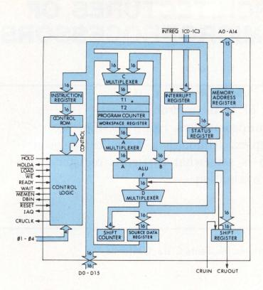
Fig 1 9900 functional block diagram. Architecture reveals absence of programmable registers and I/O port interface logic and presence of significant interrupt handling and serial-to-parallel data conversion logic. Only three registers are programmable—program counter (PC), status register (SR), and workspace register (WR). Separate nonmultiplexed data and address buses can operate at speeds up to 4 MHz but require 4-phase clock
