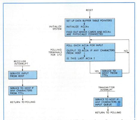
Fig 3 System software. In addition to initilization routine, software performs two simple routines: polling ACIAs for I/O and receiving interrupt to service data from host
