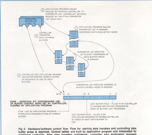
intelligent controller. After data transfers commence, controller and application program agree on allocation of data areas through buffer control word
