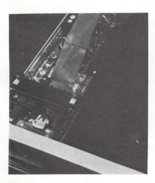
Onyx C8000 microcomputer system is pictured from above with cover removed. 10M-byte rigid disc drive (right) and 12M-byte cartridge tape drive (left) are revealed. Not shown is 4-MHz Z80A CPU board which mounts on hinged platform and covers drives and power supply
