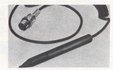
High performance model LTP-105 features high emi immunity and high scan rate response. A slim body dimension—0.625" (1.59 cm) OD and 6" (15 cm) long—with tapered narrow head permits easy aiming on the target surface. A single 5-V power supply is required. Max scan rate responses up to 5000 cm/ms are typical. Elimination of mechanical switching in the circuit increases performance life. **Photobell Co,** 162 5th Ave, New York, NY 10010.
