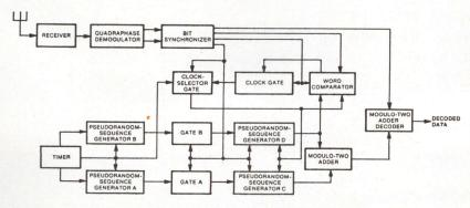
Fig 2 Receiver/decoder is controlled by a timer set identically to that in transmitter/encoder, and uses identical shift registers
