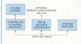
FAST-3805 semiconductor disc holds up to 72M bytes and two controllers. Internally system is organized around SBC-86 computer and Multibus. Optional RS-232 port allows attachment of remote configuration console
