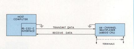
Fig 1 Host to multiplexer link. System shows link via two transmission lines. Up to 64 terminal lines may operate in any mix of baud rates from 300 to 9600 in groups of 8 per I/O module
