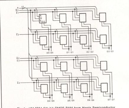
Fig 1 HM-6564 64k-bit CMOS RAM from Harris Semiconductor. Array consists of 16 4k x 1 static RAMs sharing common address bus (A). Write enables  $(\overline{\mathbb{W}1}, \overline{\mathbb{W}2})$  each address subset of eight RAMs. Chip enables  $(\overline{\mathbb{E}1}, \overline{\mathbb{E}2}, \overline{\mathbb{E}3}, \overline{\mathbb{E}4})$  each address four RAMs. Data I/O lines (D0, Q0 through D7, Q7) service one pair of RAMs each
