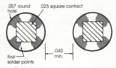
How it's done: you saw off the square .025" tail and push it through a .057" round hole in the PC board. You get only 4 contact points for solder. And there's room for only one tracing between holes. But, so what...it works.
