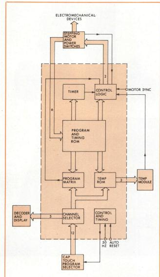
Fig 3 System architecture for washing machine CMOS controller.<sup>5</sup> Logic is simplified by having up to 64 program steps arranged sequentially, with specific time value assigned to each
