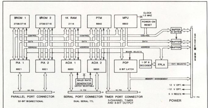
Sys-68 single-board computer from Synetic Designs is a 6800 based system that is configurable with additional memory, offboard modules, and software library to serve OEM industrial control and instrumentation applications. System cards require only 5-V power; P/ROM chips (2708) and interface modules (RS-232-C) require  $\pm$ 12-V supplies
