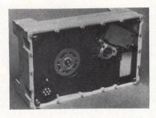
Vacuum sealed portion of Micropolis Corp's 8" rigid disc drive as seen from bottom (through transparent enclosure for demonstration purposes). Available with 1, 3, or 5 recording surfaces, units offer up to 45M bytes of unformatted storage capacity in overall enclosure about 80% smaller than existing 14"
