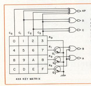
Multiplexed keyboard encoder circuit. Three transistors convert current drawn from column line encoder gate inputs into current drawn from row line encoder gate inputs. Four 2-input NAND gates encode key position in 4-bit word One 4-input (ABCD). NAND gate tests for any column line grounded and generates pressed (KP) signal
