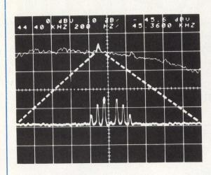
Display generated by 7530A presents at all times entire spectrum, analysis window width and starting frequency, window only zoomed to full width, and all parameters of every element in either spectrum in direct reading calibrated alphanumeric readouts
