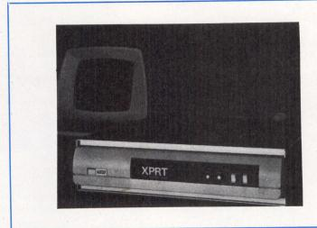
XPRT X.25 protocol tester. User has control of functions, protocol parameters such as window size and time-out values, frame and packet parameters, data generation, and error condition generation. Unit will flag any errors caused by device under test
