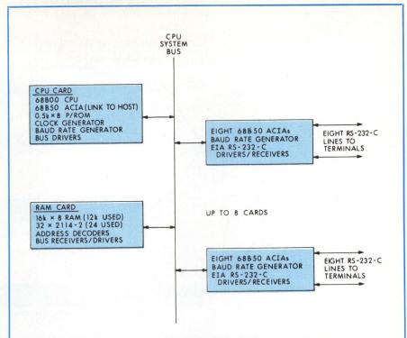
Fig 2 Internal architecture. Interface to host and system program memory are mounted on CPU board. For maximum load, 12k RAM is required; for 32 terminals 8k RAM is sufficient. System software determines how many terminal boards and ACIAs are physically connected; thus, boards or ACIA chips can be removed for maintenance without disabling entire system
