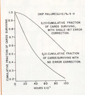
Fig 1 Cumulative fraction of cards surviving without and with single-bit error correction. Significant increase in cumulative fraction of cards surviving results when single-bit error correction is used
