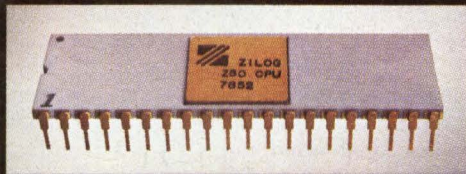
Ramtek's Micrographic Terminal is controlled by a powerful Zilog Z-80 with 28K bytes of PROM and 16K bytes of RAM.
