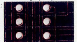
A typical example of the circuit density achievable with Multiwire circuit boards.
