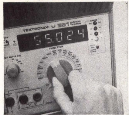
Measurement display functions of portable 851 digital tester are selected using single multiposition switch. Color-coded bands around its periphery distinguish functions involving three channels and identify them with related threshold setting functions
