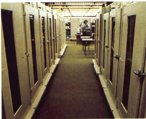
Temperature chambers stress computers to isolate marginal components. Computers are continuously tested during 72-hour burn-in at 50°C. Any error starts the test over from the beginning. To further stress the computer, power is cycled on and off approximately 2000 times during test.
