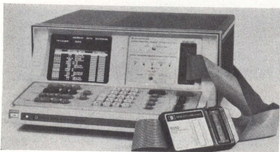
Microprocessor - controlled Logic State Analyzer for 8080 or 6800 microprocessor systems traces and displays memory transaction after memory transaction in its own mnemonics. Instrument is useful for both design and production debugging
