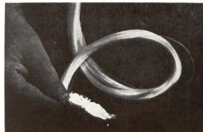
Fig. 1 Light transmission through a bundle of loose optical fibers (Corning).
