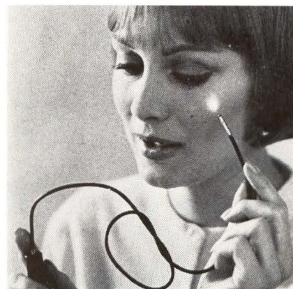
Fig. 5 Light from small flashlight travels a looped path through a light guide to dot model's cheek (DuPont)
